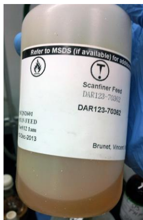
Figure 22. Discoloured Salt-Filtered Jet Fuel Sample (ideally, this sample should be clear and colourless)
