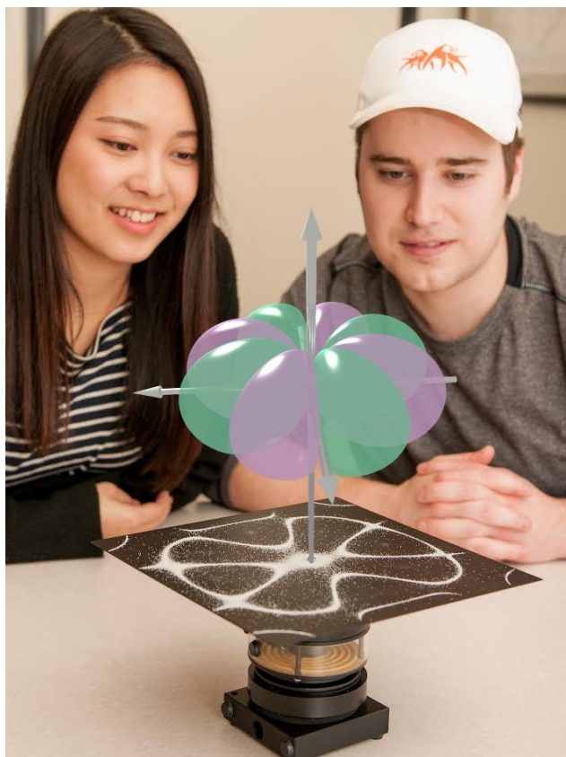
Figure 120. Chladni Plate demonstration setup featuring the characteristic nodal lines of a Chladni pattern
