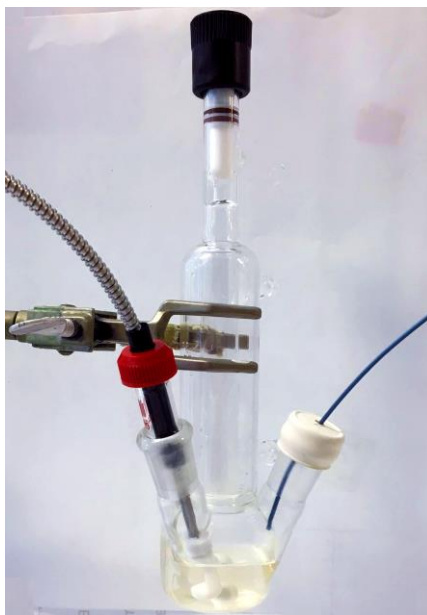
Figure 7. Photo of custom PSI flask featuring openings for a fibre optic spectrometer and PEEK tubing
