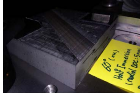
a) Half immersion up-milling with a 120^\circ fiber orientation angle
