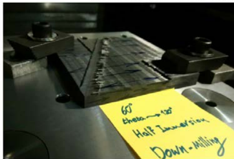
c) Half immersion down-milling with a 120^\circ fiber orientation angle
