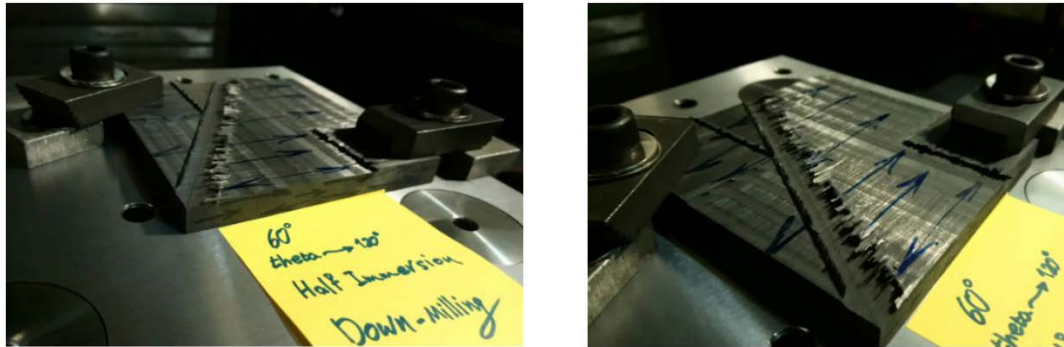
Figure 6-1: Wisps emerging from the work surface
