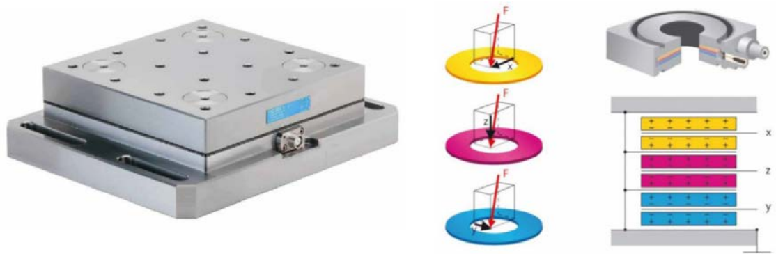
Figure 5-3: Stationary 3 component dynamometer [39]
