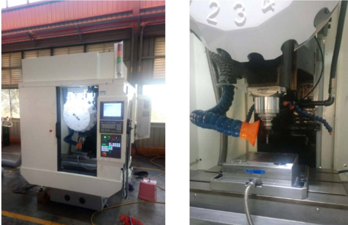
Figure 5-2: 3-Axis vertical milling machine with a special dust collector
