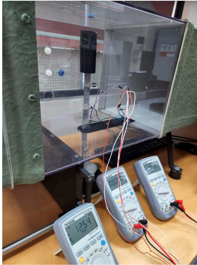
Figure 7. The experimental setup in a wind tunnel with piezoelectric sensors positioned at the tested locations.
