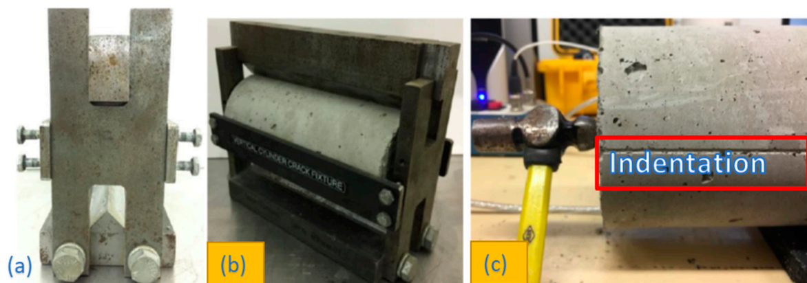
Figure 4. Setup for cracking (a) Standard Crack Inducing Jig (SCIJ) Front view (b) cylinder held in SCIJ Isometric view (c) Longitudinal Impulse Direction Setup.
