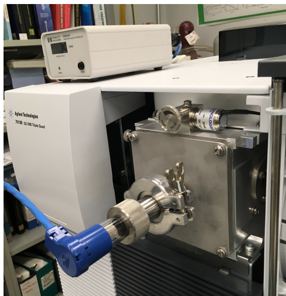
Figure 3.5.1: In-house built stainless steel flange was mounted on MS source with Hewlett Packard 59864A Ionization Gauge Controller.
