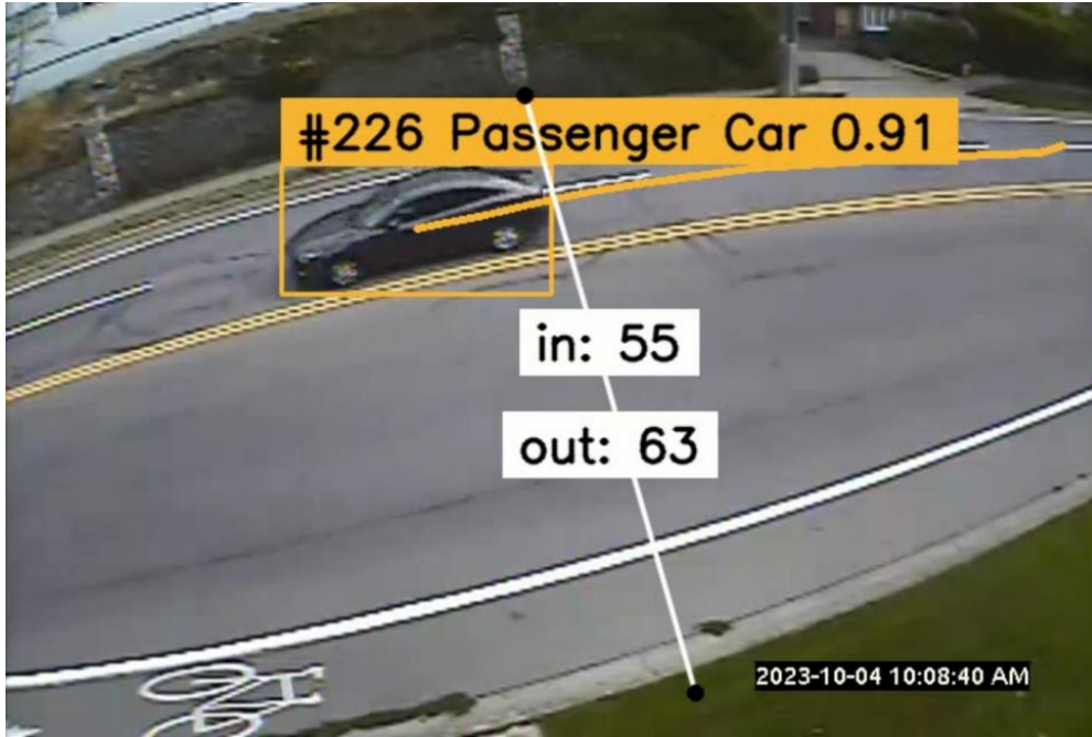
Figure S2.2. Virtual line drawn on video frame to facilitate vehicle counting.
