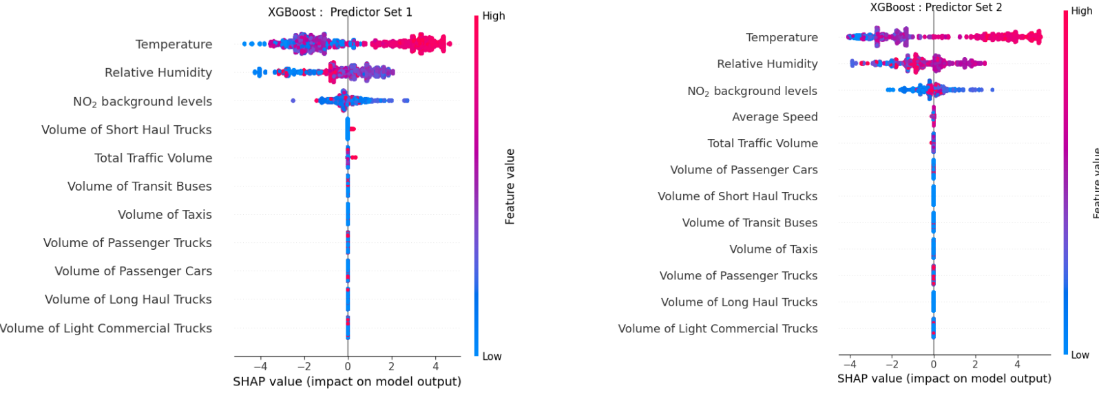
Figure S2.20. SHAP summary plot for NO 2 with XGBoost with Predictor Sets 1- 2.
