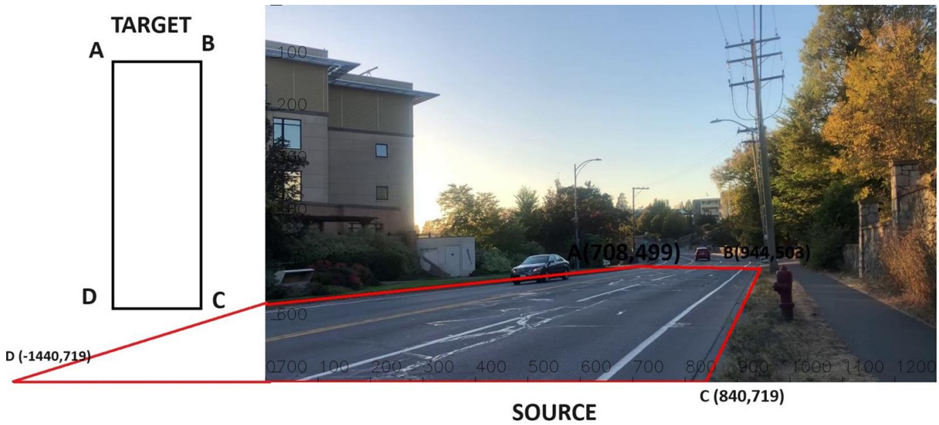
Figure S2.3. Polygon drawn on the road to estimate image coordinates of the road.
