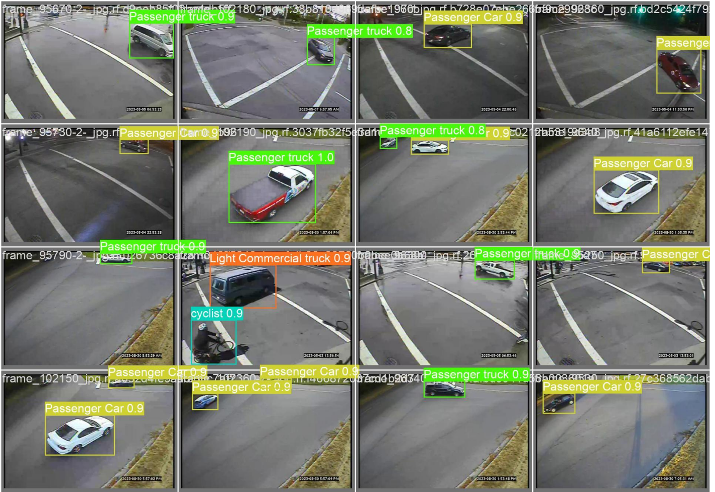
Figure S2.7. Vehicle classification by object detection model. Each frame shows the detected objects with their respective classes, along with their confidence scores represented inside the colored boxes.
