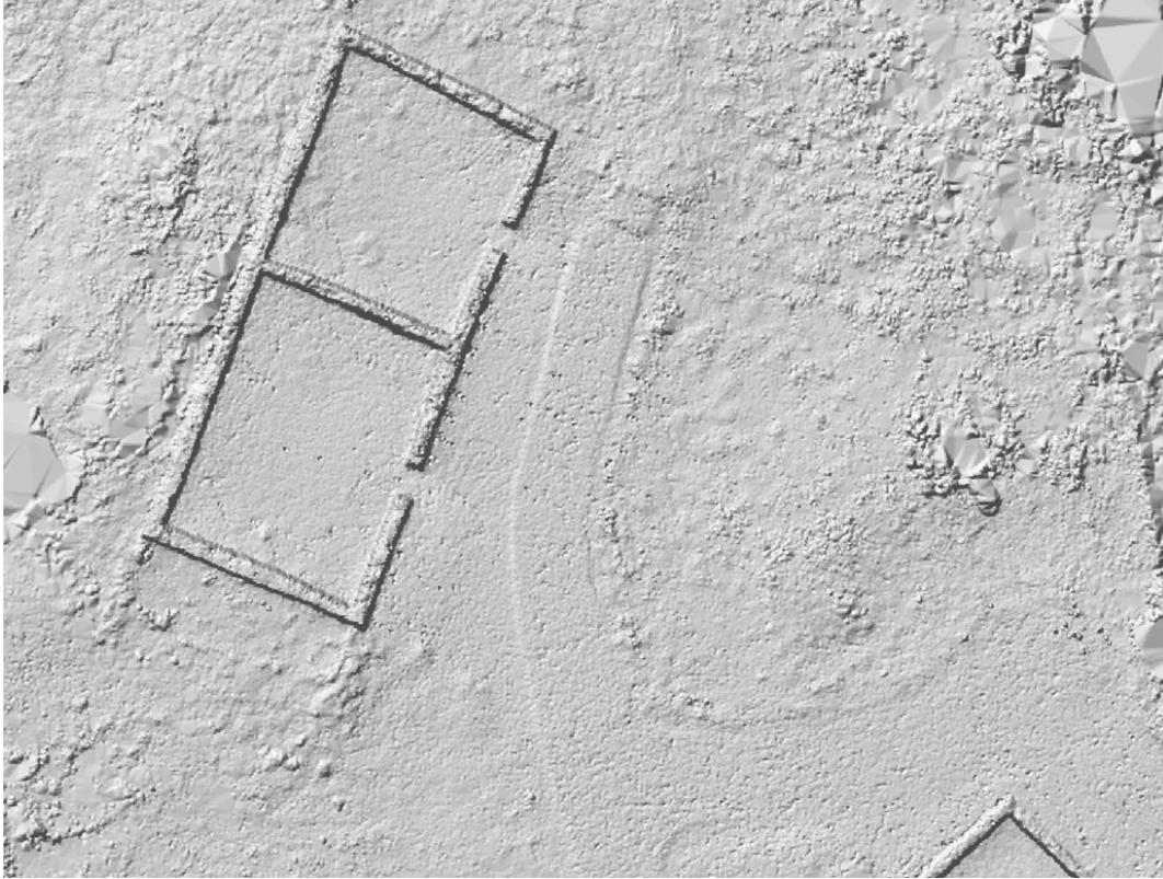
Figure 13. Hillshade Map. The smooth triangular shapes present in this scan are caused by the interpolate function for some of the areas where insufficient data points were collected during the scanning of the site. (Image created by the author for this study).
