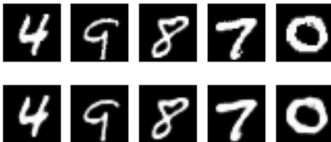
Figure 4.5: Reconstructed output of CNN autoencoder model.
