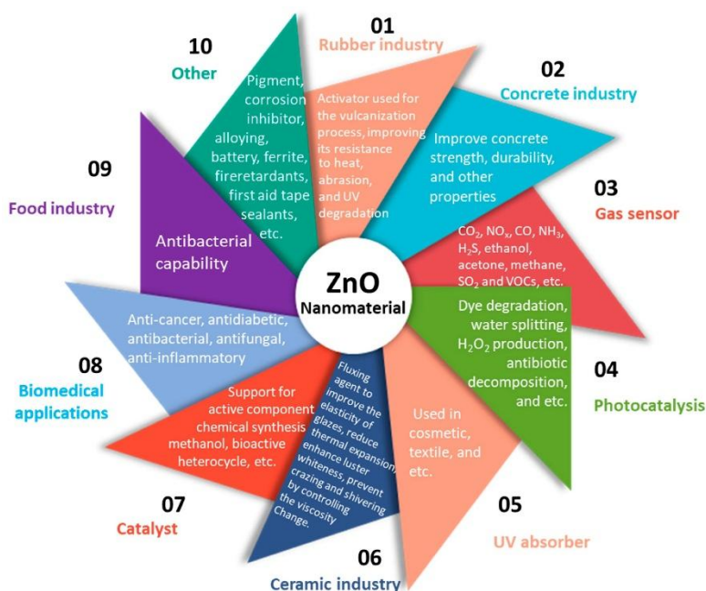
Figure 2.4: Various uses for ZnO nanomaterials and a succinct explanation of each use. Adapted from [92].
