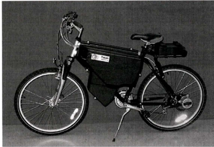
Figure 14: Palcan Fuel Cell Powered Electric Bicycle
