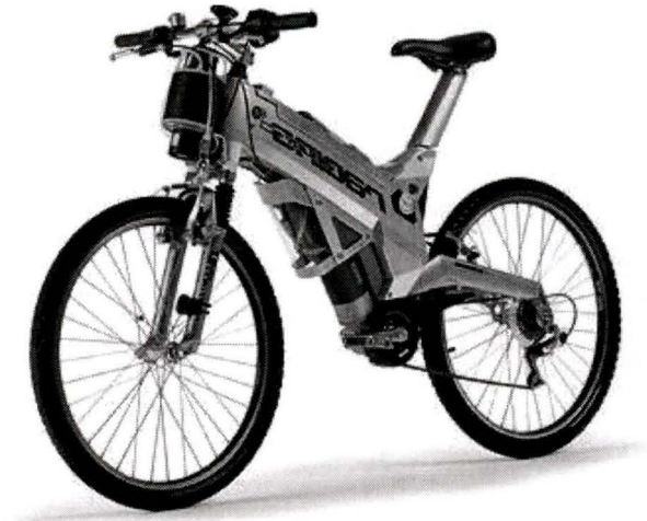
Figure 12: Aprilia ENJOY Fuel Cell Powered Electric Bicycle Prototype with Manhattan Scientifics NovArs PEM Fuel Cell Power System [19]
