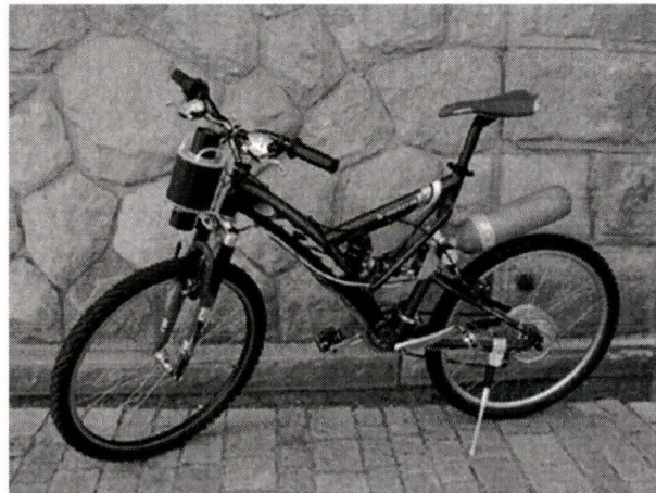
Figure 11: HYDROCYCLE™, Manhattan Scientifics Fuel Cell Powered Concept Bicycle [21]
