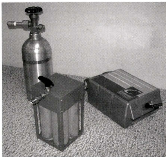
Figure 13: Palcan Metal Hydride Hydrogen Containment Shown in Middle (Compressed Hydrogen Container on Left and 24 V Sealed Lead Acid Battery Pack on Right)
