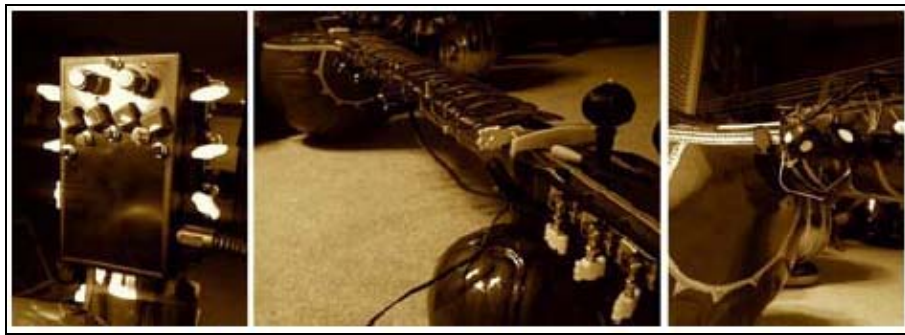
Figure 3.7. ESitar controller head, neck and thumb sensor
