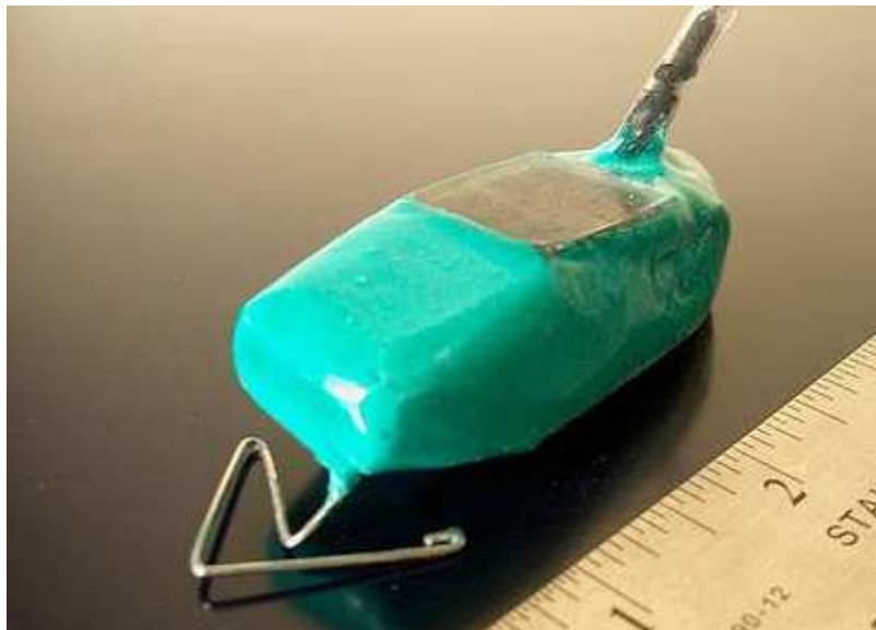
Figure 2.1: Argos avian backpack PTT transmitter [3]
