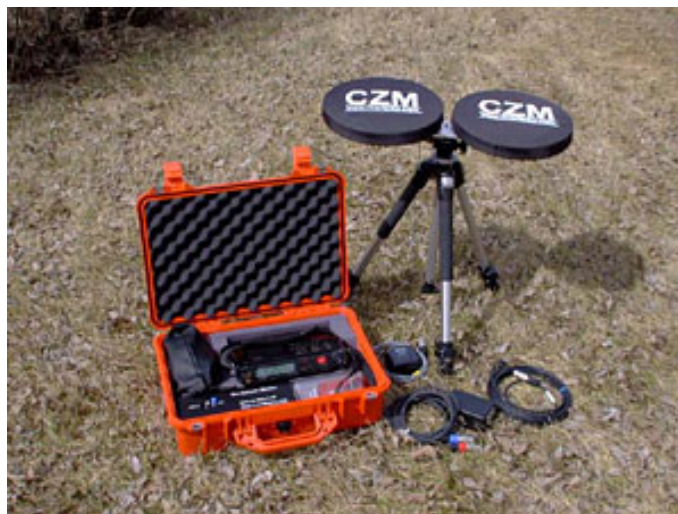
Figure D.3: An image of the CZM microphone, used to efficiently collect a stereophonic field of sound but with the ability to amplify distant sounds.
