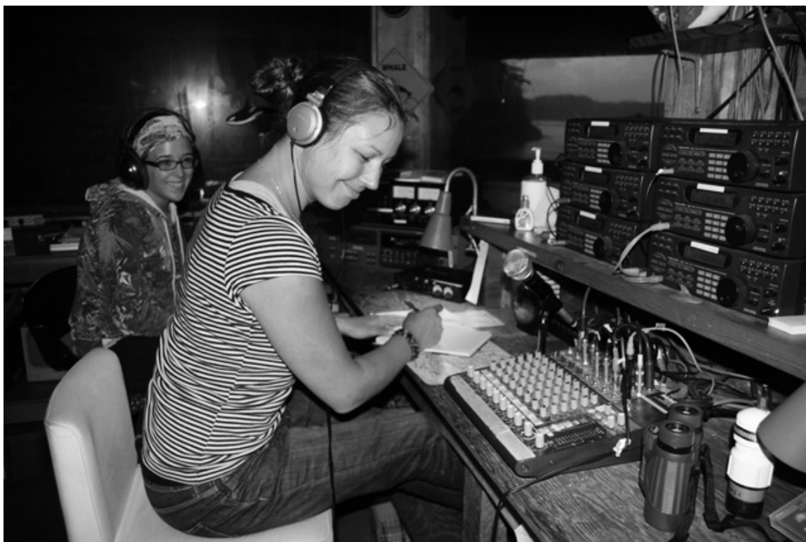
Figure 1.8: A photograph showing the inside of the OrcaLab research station, with a research assistant taking notes in a lab book as she listens to hydrophones and adjust a multi-track mixer. Other equipment that can be seen are VHF radios, binoculars, audio and Digital Audio Tape (DAT) tape recorders and a microphone for making voice notes. On the front wall is a little sign that has arrows for North and South to help orient new summer research assistants. Photo credit OrcaLab.
