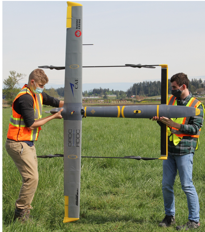
Figure 2.5: Mini-E 5050A prototype during a pre-flight IMU calibration.
