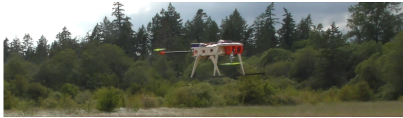
Figure 2.19: Test tri-rotor during outdoor flight testing.
