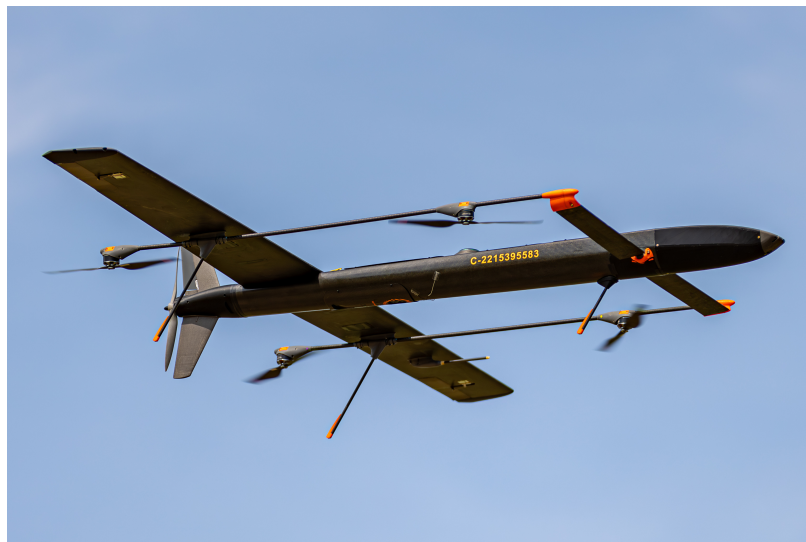
Figure 2.6: Mini-E 5050B in the VTOL phase during flight testing.
