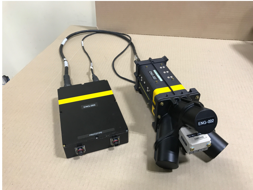
Figure 2.1: CAE Magnetic Anomaly Detection sensor (MAD-XR).
