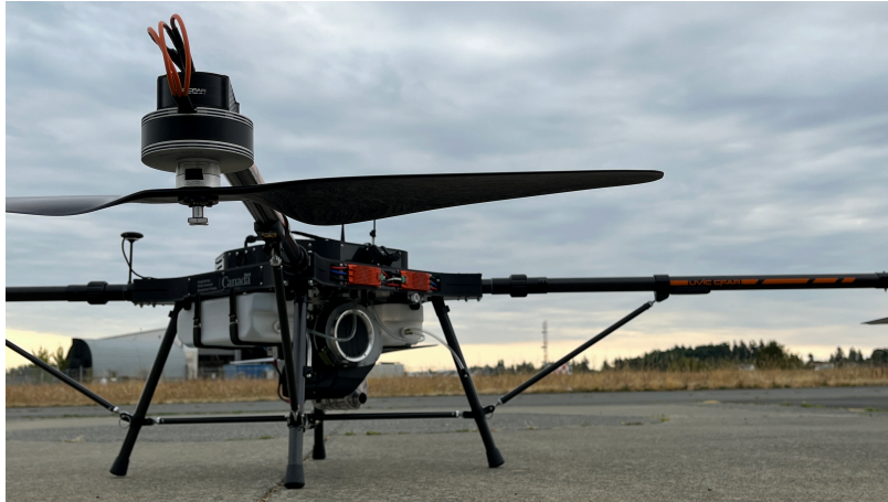
Figure 2.8: MIMIQ vehicle configured with a series ICE hybrid system.
