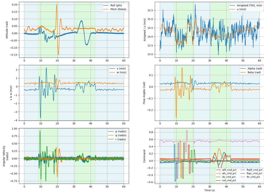
Figure 6.23: MPC test for roll attitude doublet with doublet validation and PX4 handovers.
