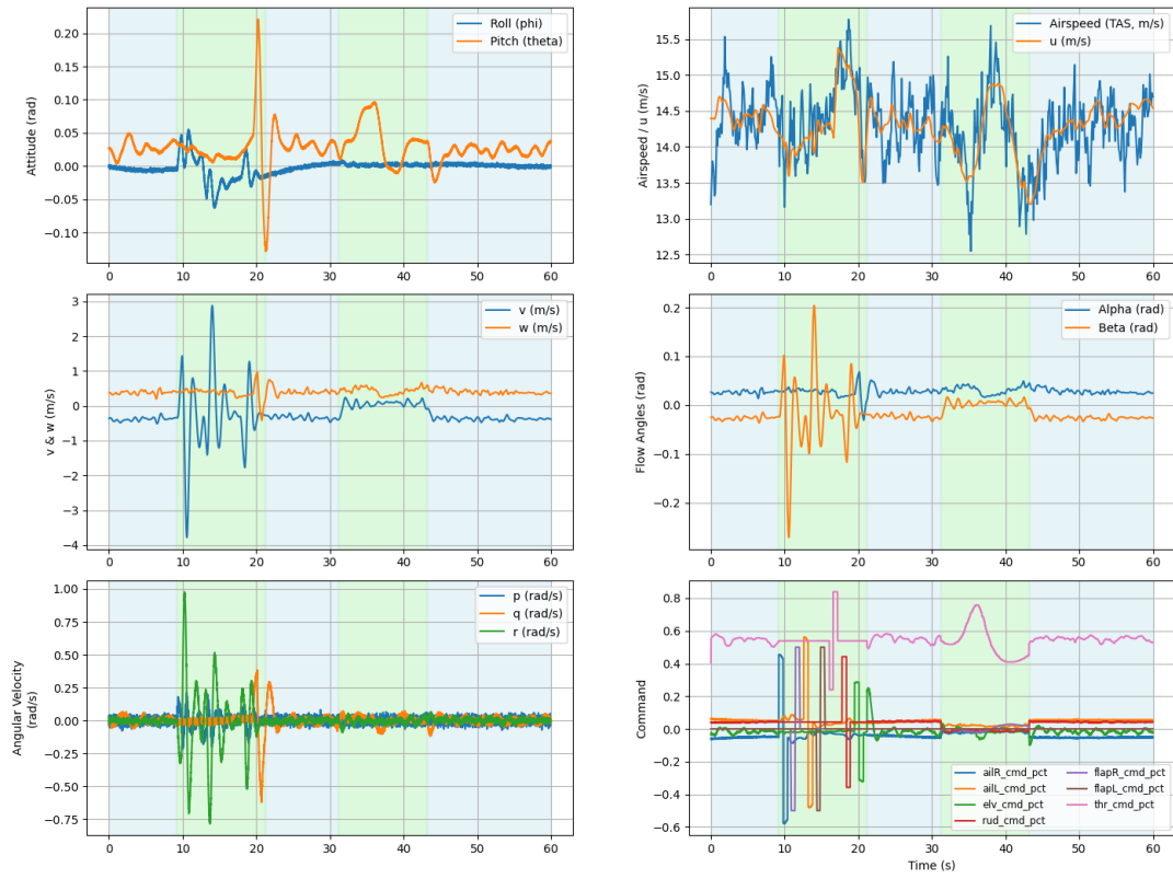
Figure 6.25: MPC test of pitch attitude with doublet validation and PX4 handovers.
