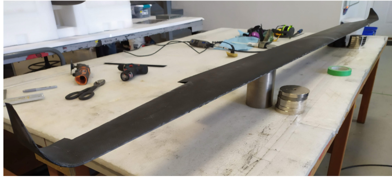
Figure 2.11: Full-scale Eusphyra wing under fabrication for structural testing.
