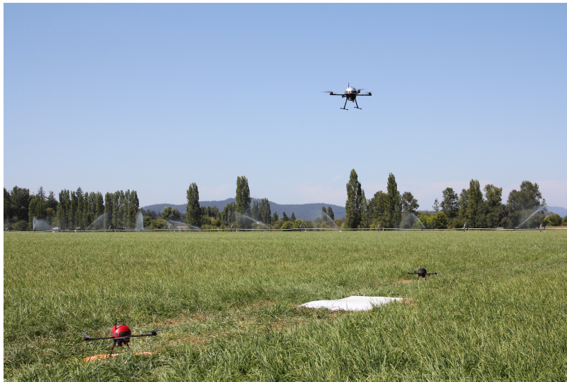
Figure 2.9: Three Tarot 650 UAVs taking off for a multi-agent flight coordination demonstration.
