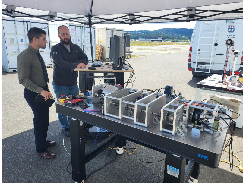
Figure 2.7: Hybrid research test bench evaluating a parallel ICE configuration.
