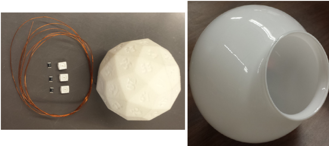
Figure 3.2: The parts used for the source: (Left) A 60-sided polyhedral die, 40 gauge enamel coated wire, 470 nm surface mount LEDs, and 270 \Omega resistors; (Right) the diffusing sphere.
