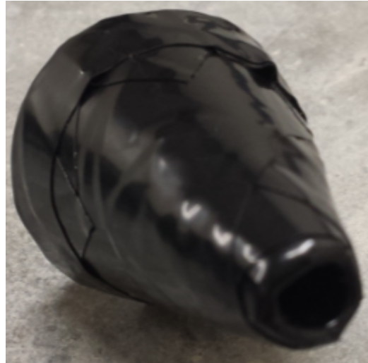
(b) The conical cap used to calibrate each LED.
