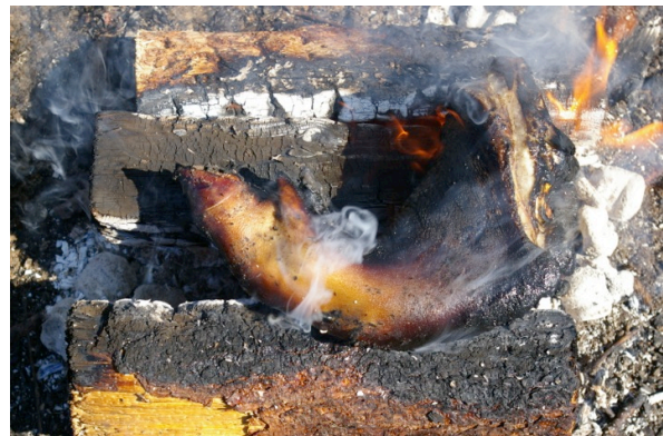
Image 10: Specimen 1. Specimen temperature: 379°C. Fire temperature: >900°C. Time: T+23. Efford 2016.
