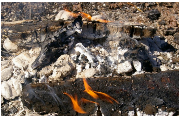
Image 4: Specimen 1. Specimen temperature: 650.2°C. Fire temperature: >900°C. Time: T+60. Efford 2016.
