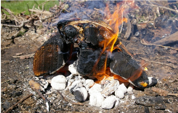
Image 10: Specimen 2. Specimen temperature read 259.5°C. Time: T+10. Efford 2016.
