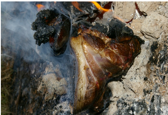
Image 6: Specimen A. Specimen temperature: 461.7C. Fire temperature read over 900° C. Efford 2015.
