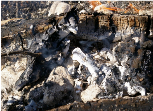
Image 14: Specimen 2. Specimen temperature: 649.1°C. Fire temperature: >900°C. Time: T+69. Efford 2016.
