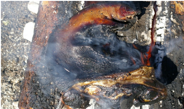
Image 13: Specimen 2. Specimen temperature: 553.9°C. Fire temperature: >900°C. Time: T+39. Efford 2016.
