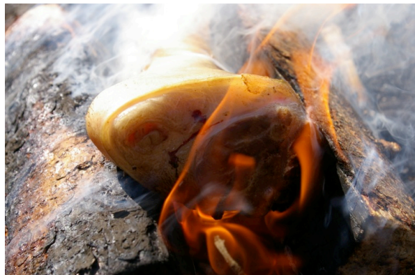
Image 6: Specimen 1. Specimen temperature: 235.6°C. Fire temperature read >900°C. Time: T+14. Efford 2016.
