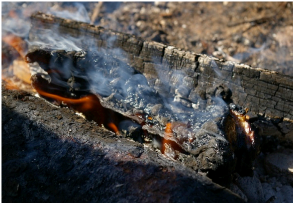
Image 11: Specimen 1. Specimen temperature: 502.7°C. Fire temperature: >900°C. Time: T+30. Efford 2016.
