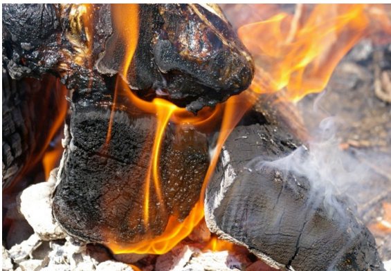
Image 10: Specimen 1. Specimen temperature: 491.1°C. Fire temperature: >900°C. Time: T+10. Efford 2016.
