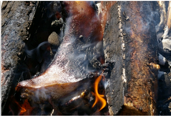
Image 12: Specimen 2. Specimen temperature: 480.2°C. Fire temperature: >900°C. Time: T+24. Efford 2016.
