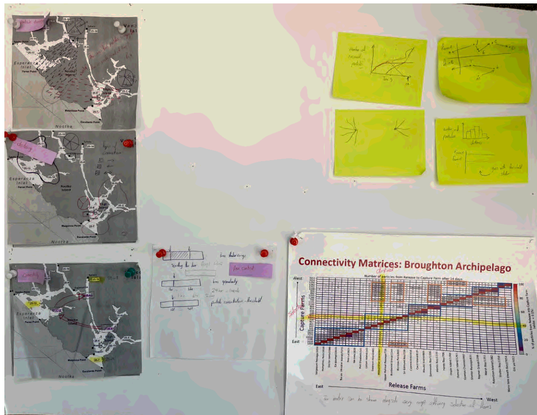
Figure 3.5: Low-fidelity paper prototype used as a shared artifact during expert walkthrough. The board aggregated candidate components (map, matrix, time and threshold controls, and alternative encodings) to support comparison of design directions before implementation.
