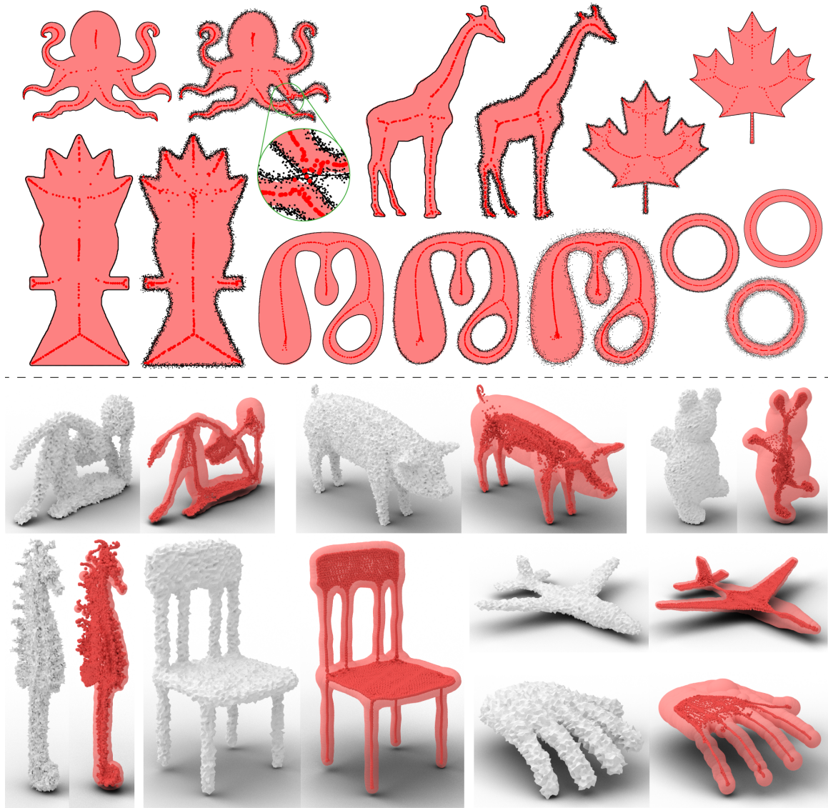
Figure 4.1: A gallery of LSMAT results with varying levels of noise on shapes with complex topology and varying feature size. In the callout for the octopus, notice how the MLS kernel overlaps nearby surfaces, yet the algorithm can cope by producing erroneously located medial spheres with a zero radii.
