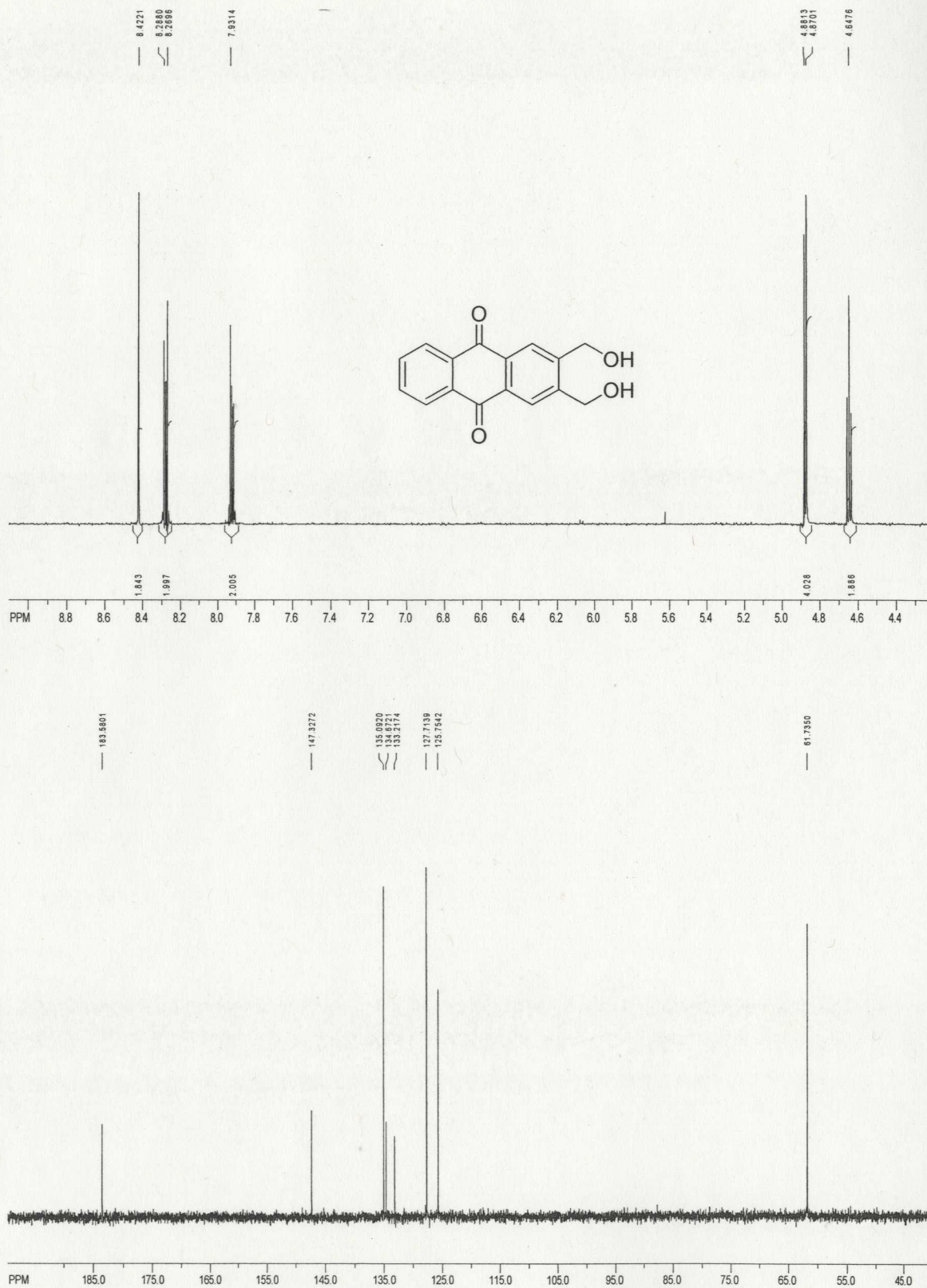
Figure A - 7 ^1\text{H} (top) and ^{13}\text{C} NMR (bottom) for 2,3-di(hydroxymethyl)-9,10-anthraquinone (2.7) in Acetone- d_6 at 300 K.
