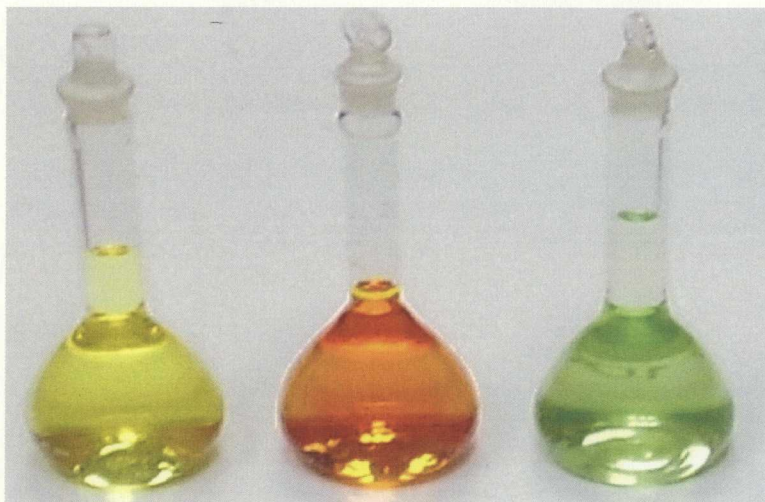
Figure 4.4 Dramatic differences in observed colors in the photolysis of 4.2 (pH 7), HMAQ (pH 7), and 4.1 (pH 1) (L to R) in 1:1 H 2 O-CH 3 CN ( \lambda_{\text{ex}} 350 nm; 15 min; argon purged). The color remained unchanged for at least a day for 4.2 and HMAQ and a few hours for 4.1 .
