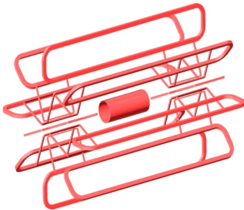
Figure 3.17: Layout of the three types of magnets used in the ATLAS detector: the solenoid in the center, the two end-cap and the barrel toroids. Figure from [74] .
