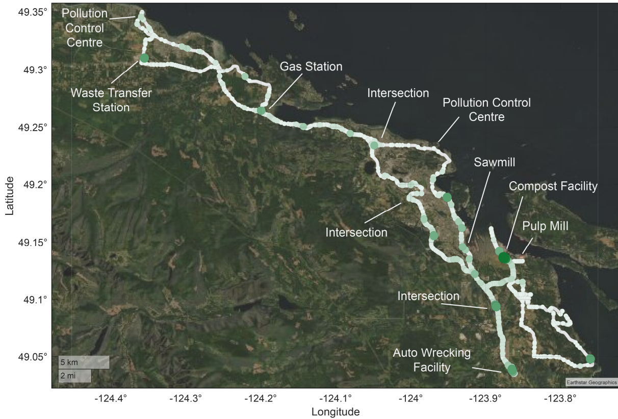
Figure 4.55: Geospatial distribution of the small oxygenated species component (Component 5 of 8) in the MCR-WALS model of the August 14, 2018 data. Larger and darker dots indicate higher signal intensities. This component was measured near many different point sources, such as the composting facility, waste transfer station, gas station, and auto wrecking facility.
