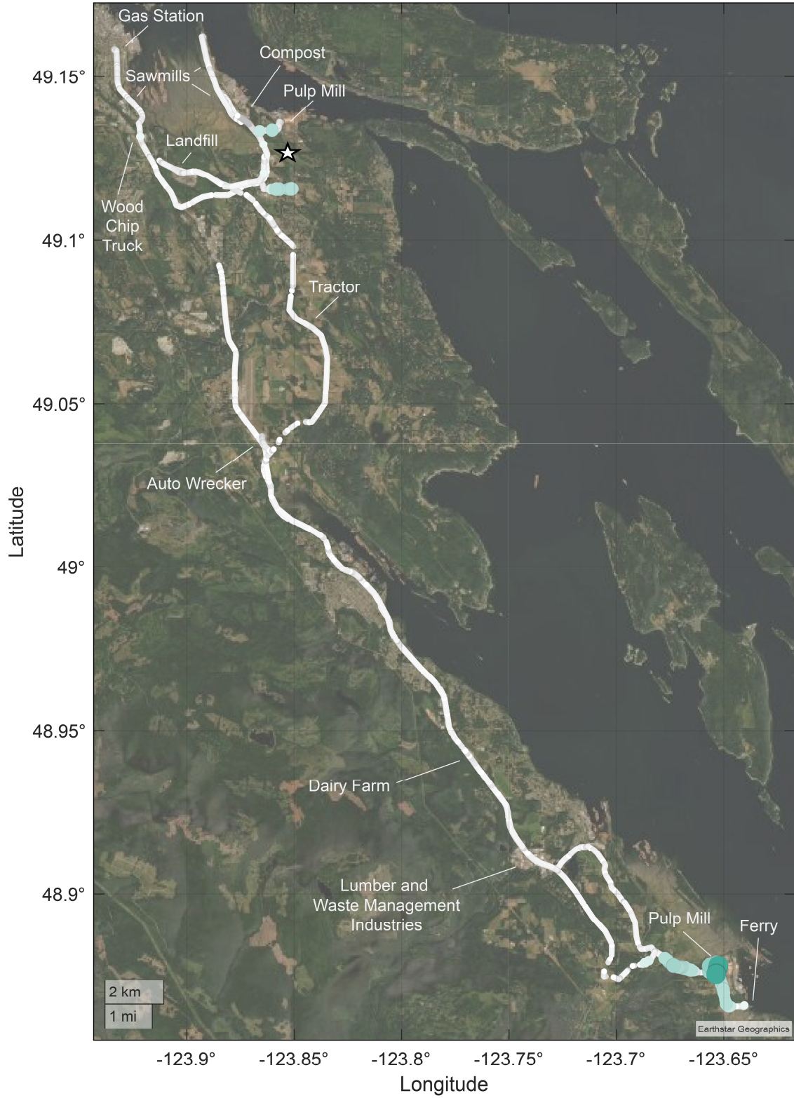
Figure 4.77: Geospatial distribution of the pulp mill emissions (Component 3 of 9) in the MCR-WALS model of the August 21 and 22, 2017 Nanaimo to Crofton data. Larger and darker dots indicate higher signal intensities. This component was measured near the pulp mills on the drive route. The white star indicates the location of the Harmac Cedar Woobank air quality monitoring station (hourly TRS measurements).
