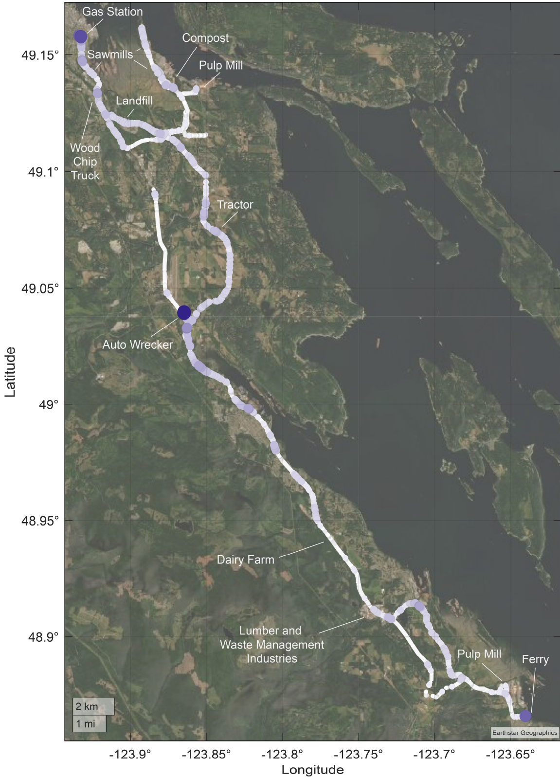
Figure 4.75: Geospatial distribution of the anthropogenic hydrocarbon emissions (Component 2 of 9) in the MCR-WALS model of the August 21 and 22, 2017 Nanaimo to Crofton data. Larger and darker dots indicate higher signal intensities. This component was measured at the ferry terminal, auto wrecker, gas station, and while driving.
