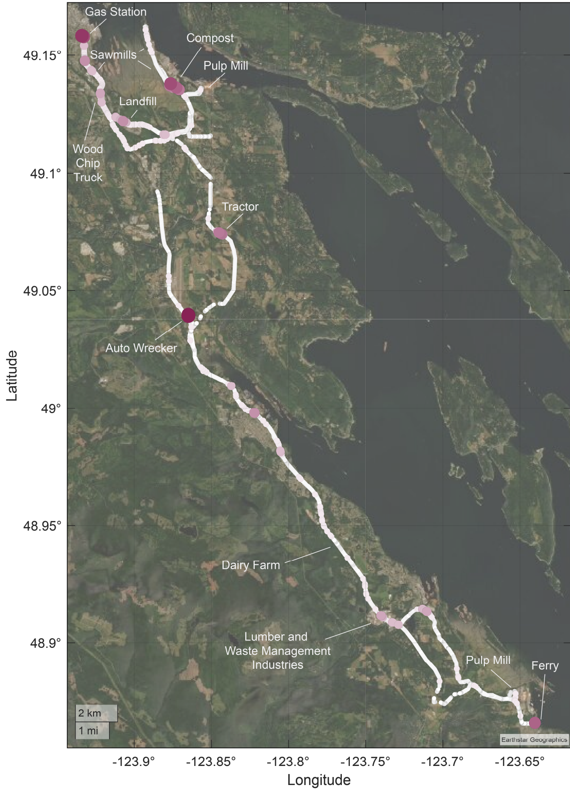
Figure 4.86: Geospatial distribution of the small hydrocarbons and oxygenated species component (Component 7 of 9) in the MCR-WALS model of the August 21 and 22, 2017 Nanaimo to Crofton data. Larger and darker dots indicate higher signal intensities. This component was measured in many locations including near the ferry terminal, auto wrecker, gas station, while passing a tractor, the compost facility, and landfill.
