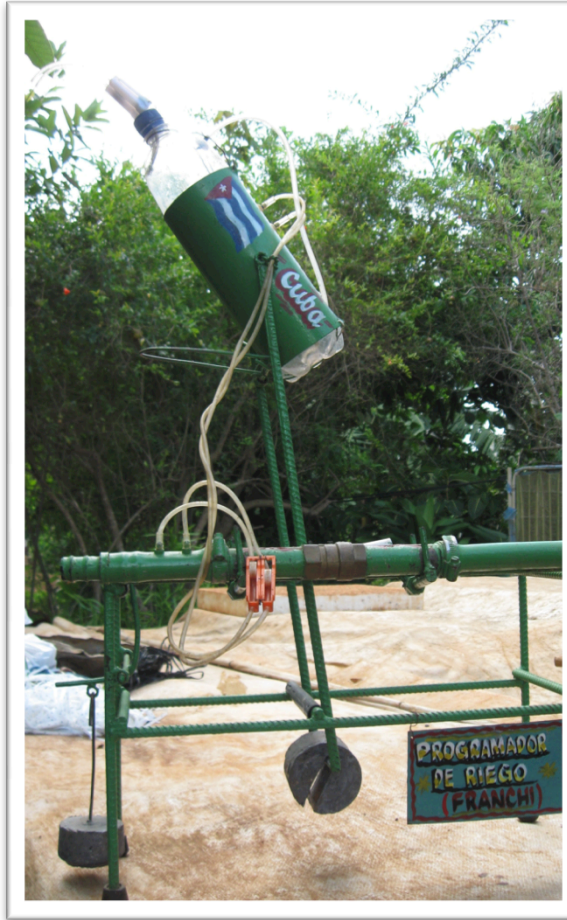
Photo 2: A homemade gravity-timed watering system that provides protection from electricity interruptions
