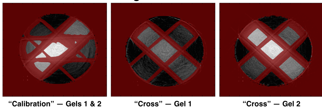
Figure 5.20: Dose distributions for the “Calibration” and “Cross” irradiation patterns with steep dose gradients cut in order to calculate calibration curves. Regions in red were not included for calibration curve calculations.
