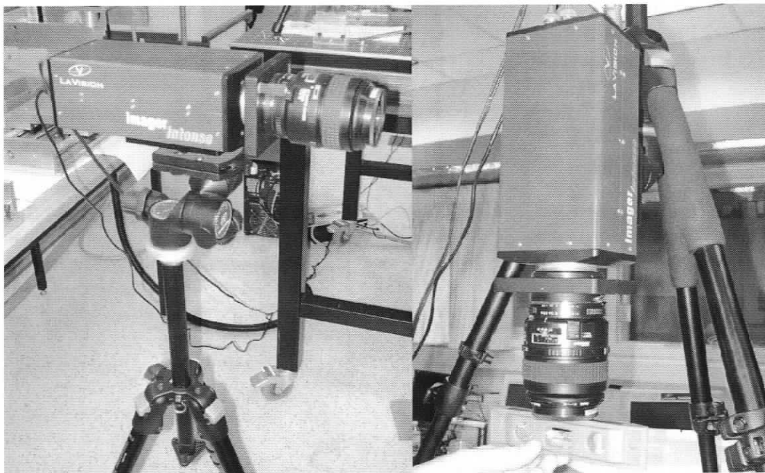
Figure 2.2-4. Horizontal (left) and vertical (right) camera set-up. For both cases cameras were aligned by means of spirit levels.
