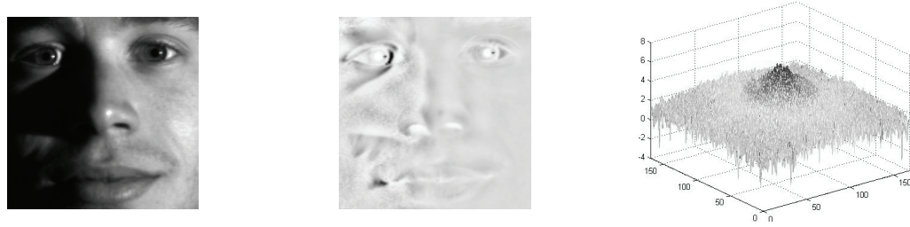
Figure 3.3. The effect of WII pre-processing: original image (left hand side), its processed counterpart (middle) and the power spectrum of the processed counterpart (right hand side).
