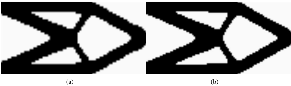
Figure 40: Optimal topologies for the 2:1 length to width ratio cantilever beam without hole and a load at the middle of the free end using various numbers of material points with a horizon size 2\Delta . (a) 80 \times 40 . (b) 100 \times 50 .
