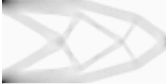
Figure 41: Strain energy density representation using scaled colors.
