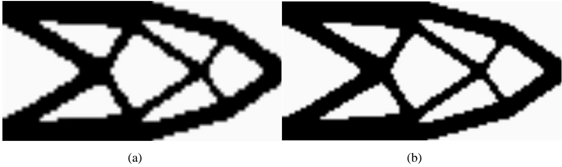
Figure 39: Optimal topologies for the 2:1 length to width ratio cantilever beam with hole and a load at the middle of the free end using various numbers of material points with a horizon size 2\Delta . (a) 80 \times 40 (iteration 1302) with the conical bond function and the projection operator. (b) 100 \times 50 (iteration 1203) with the conical bond function and the projection operator.
