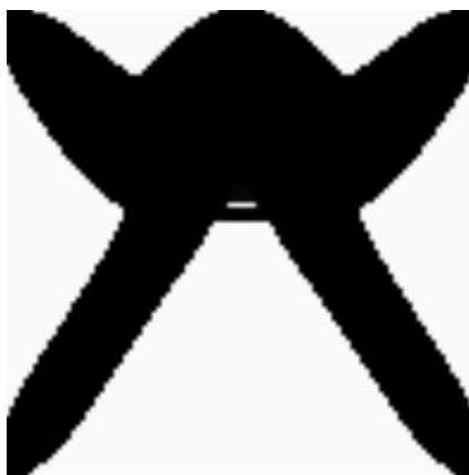
Figure 43: Optimal topology for a 100 \times 100 plate hinged from all corners with a horizon size 2\Delta (iteration 501).
