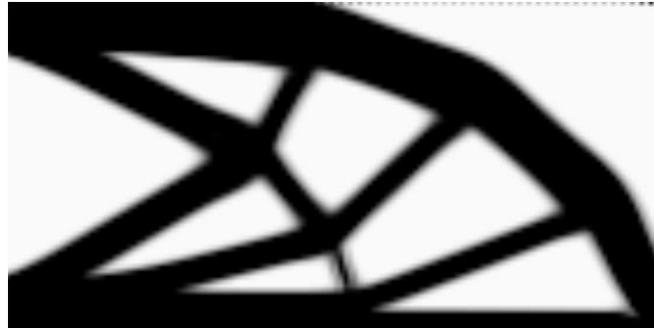
Figure 33: Optimal topology for 140 \times 70 material points with a horizon size 2\Delta when load is at the bottom corner with the conical bond function and without the projection operator (iteration 1638).
