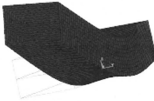
Figure 2.13 ANSYS active spar model showing the maximum load response
