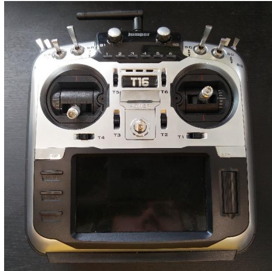
Figure 24: Jumper T16 UAV Pilot Console. Control sticks are used to control aircraft movement, while switches and knobs can be configured based on requirements.
