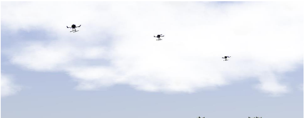
Figure 25: Simulated Line Formation using FDM of experimental aircraft in Gazebo. The center aircraft is leading the horizontal line formation towards image left.
