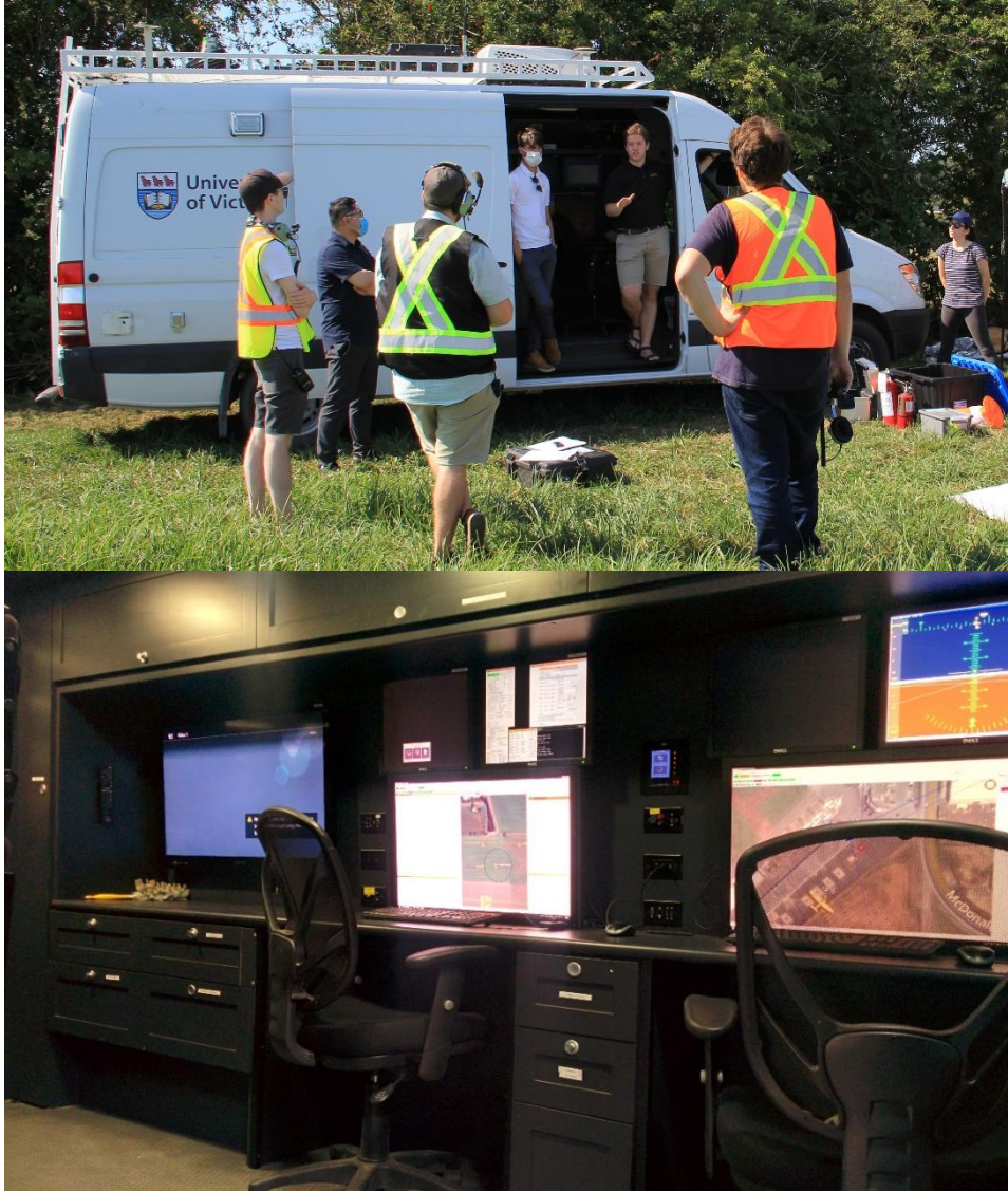
Figure 23: CfAR Ground Station Van. In use during a flight test (top) and, showing interior with two desktop computers (bottom).
