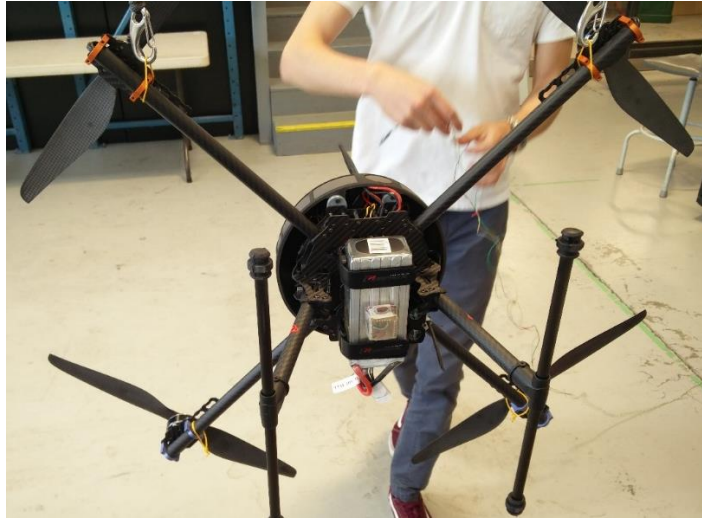
Figure 20: Bifilar Pendulum inertia test. Aircraft is supported from two of its motor mounts, using long cables, facing down, allowing it to rotate about the roll axis (axis pointing directly forward from the center of mass).
