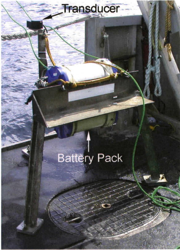
Figure 3.3. Aluminum tripod on the deck of MSV John Strickland following recovery on April 21, 2006. The acoustic transducer was located 0.5 meters above the seabed.
