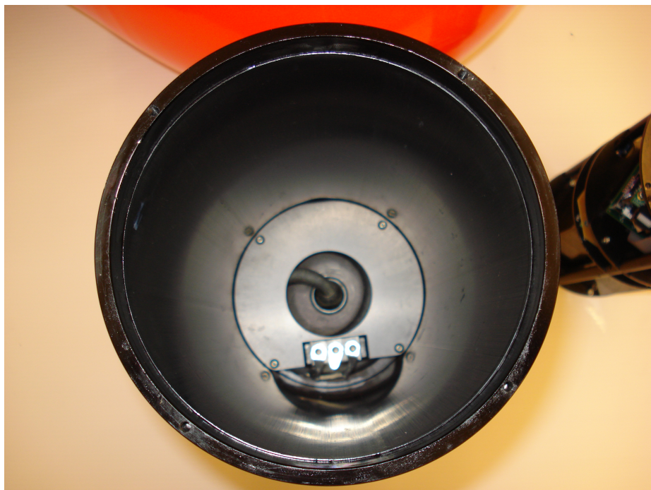
Figure A.4: Photograph showing the blind stab connectors at the bottom of the UGPS satellite pressure vessel. These connectors allow the majority of the satellite hardware to be removed while the projector stays fixed to the housing.
