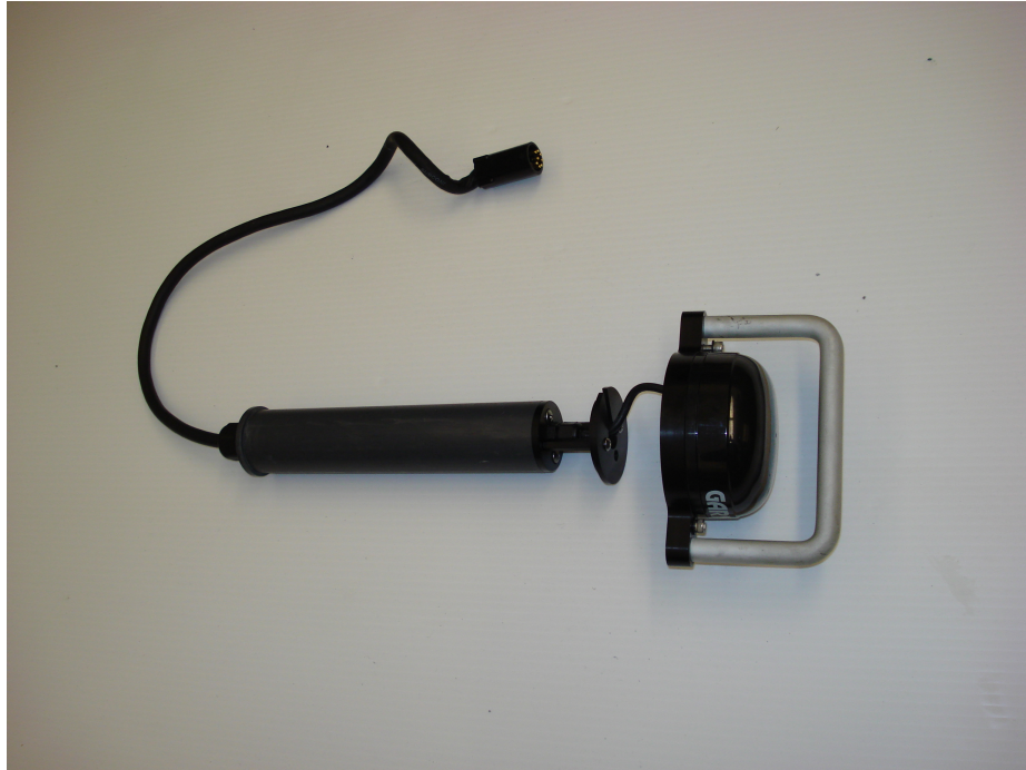
Figure A.6: Photograph of the wireless Ethernet module that is mounted inside the orange float of the UGPS satellite. The Garmin GPS is mounted to the top of the float.
