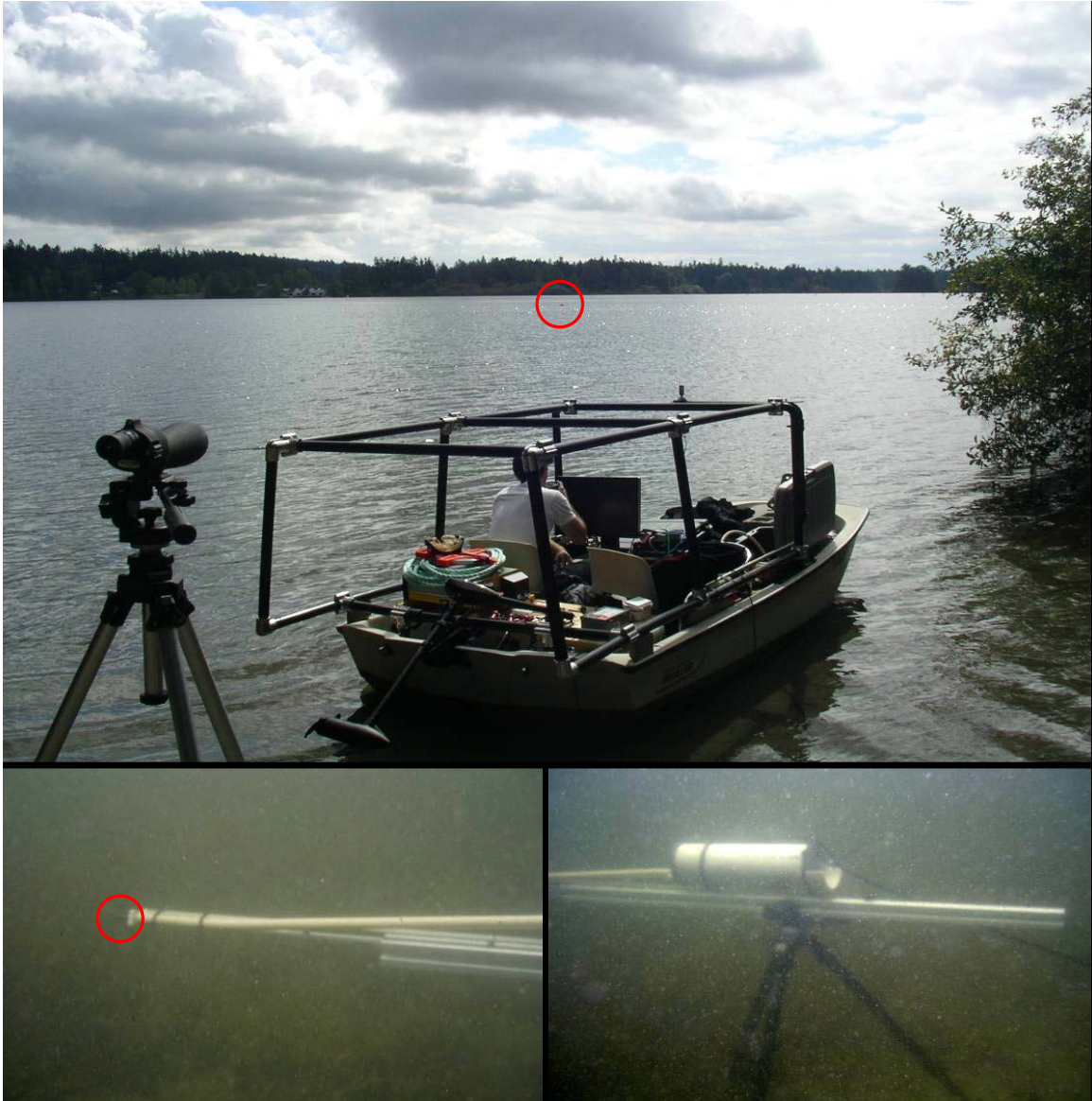
Figure 5.7: Top: Photograph of the spotting scope directed at the UGPS satellite (shown in the center of the red circle) in the distance. Bottom: UGPS receiver mounted on the underwater tripod. The hydrophone is identified by the red circle.
