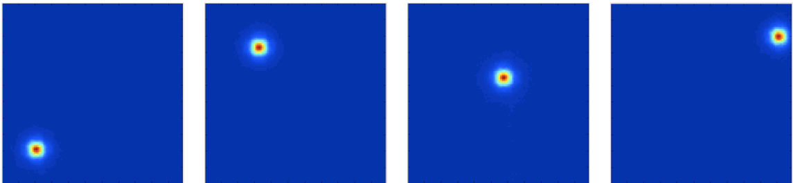
Figure 2.2: Top view of four influence functions for a 1024-actuator MEMS DM.
