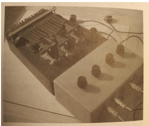
Figure 7.1: Thumb piano with electromagnetic drivers by Dan Wilson
