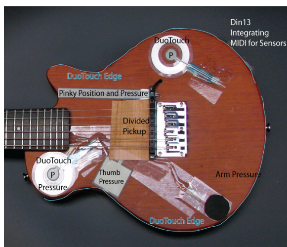
Figure 6.3: Adrian Freed's augmented guitar prototype
