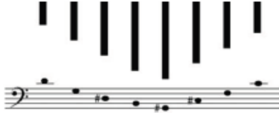
Figure 3.15: tine layout/approx. A=440
