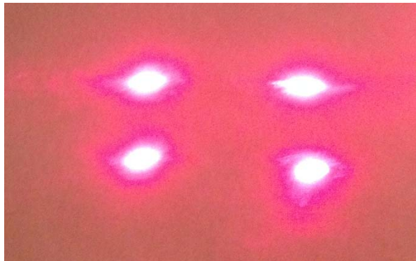
Figure 4.5 Four parallel laser projection on slope bottom with tilted camera.
