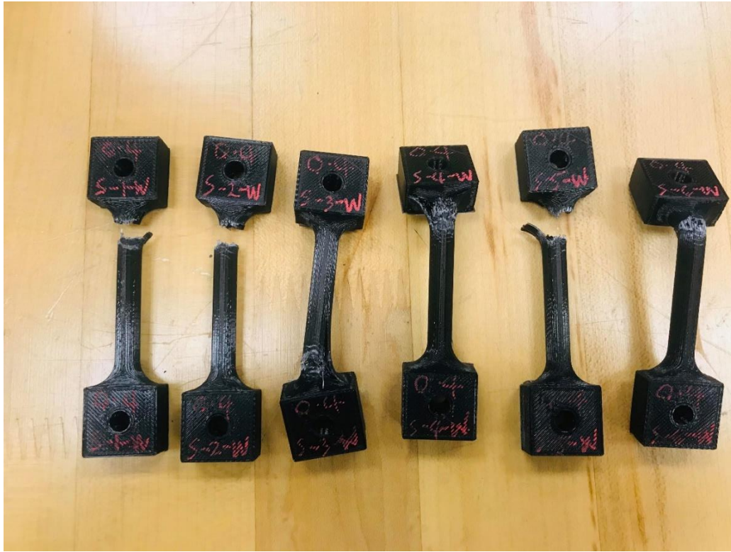
Figure 28: Side printed; Wide-side clamped samples after bending testing
