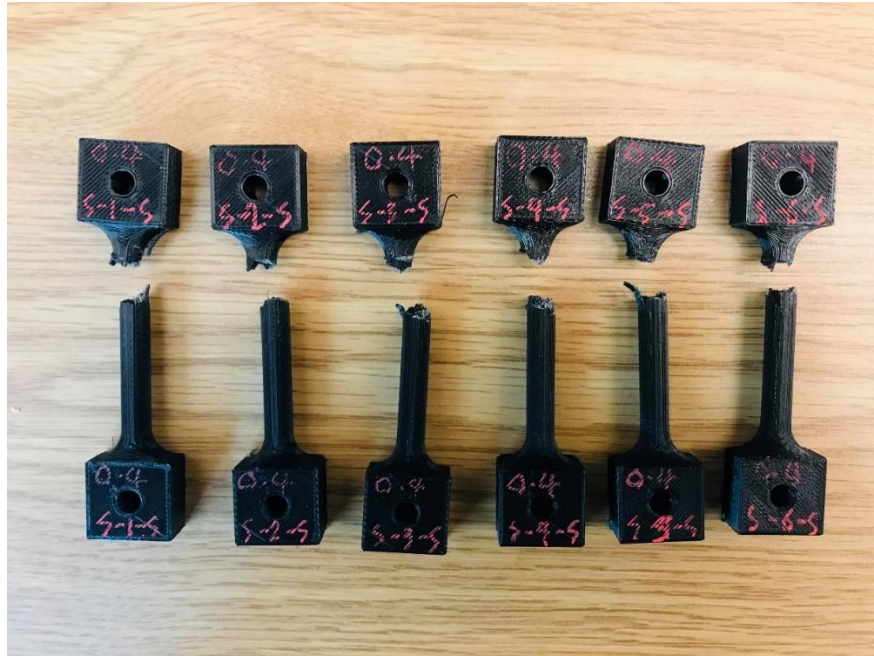
Figure 33: Side printed; Short-clamped samples after bending test
