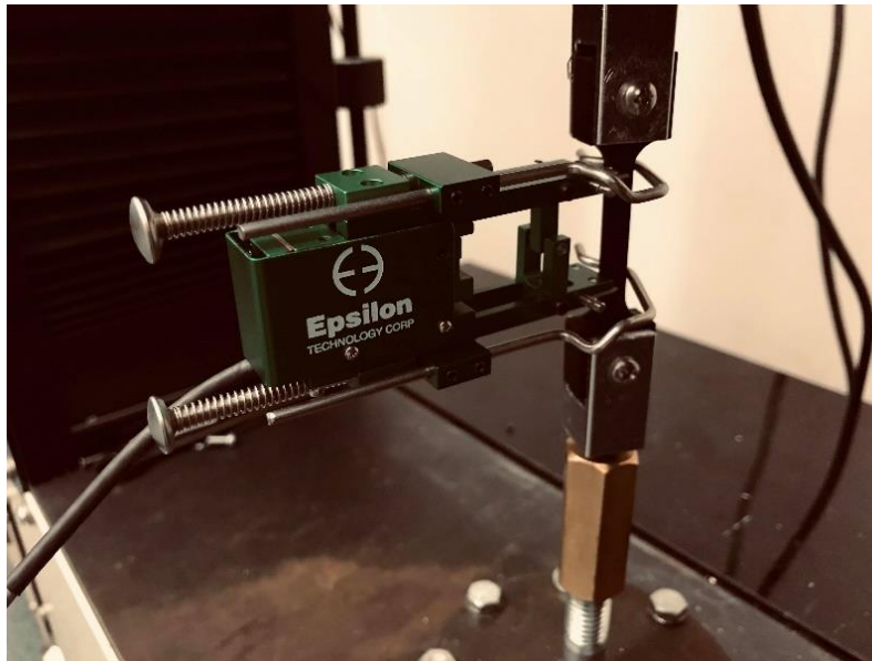
Figure 12: Extensometer attached before testing
