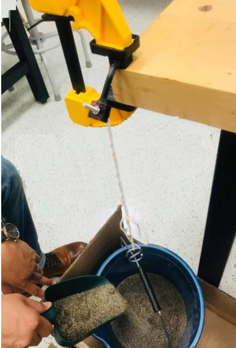
Figure 26: Pouring of sand into the bucket as load
