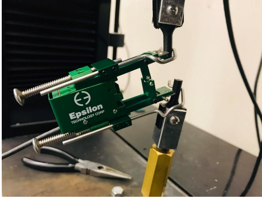
Figure 13: Extensometer position after the fracturing of the specimen
