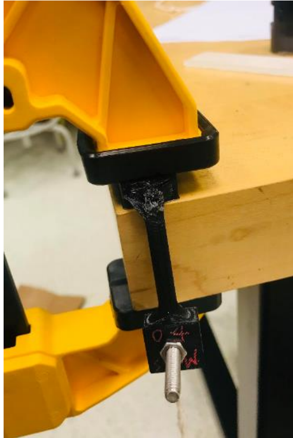
Figure 27: Specimen after loading
