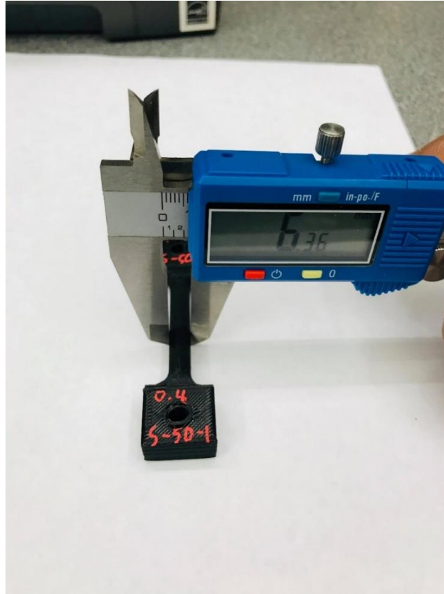
Figure 9: Measuring the diameter of the samples
