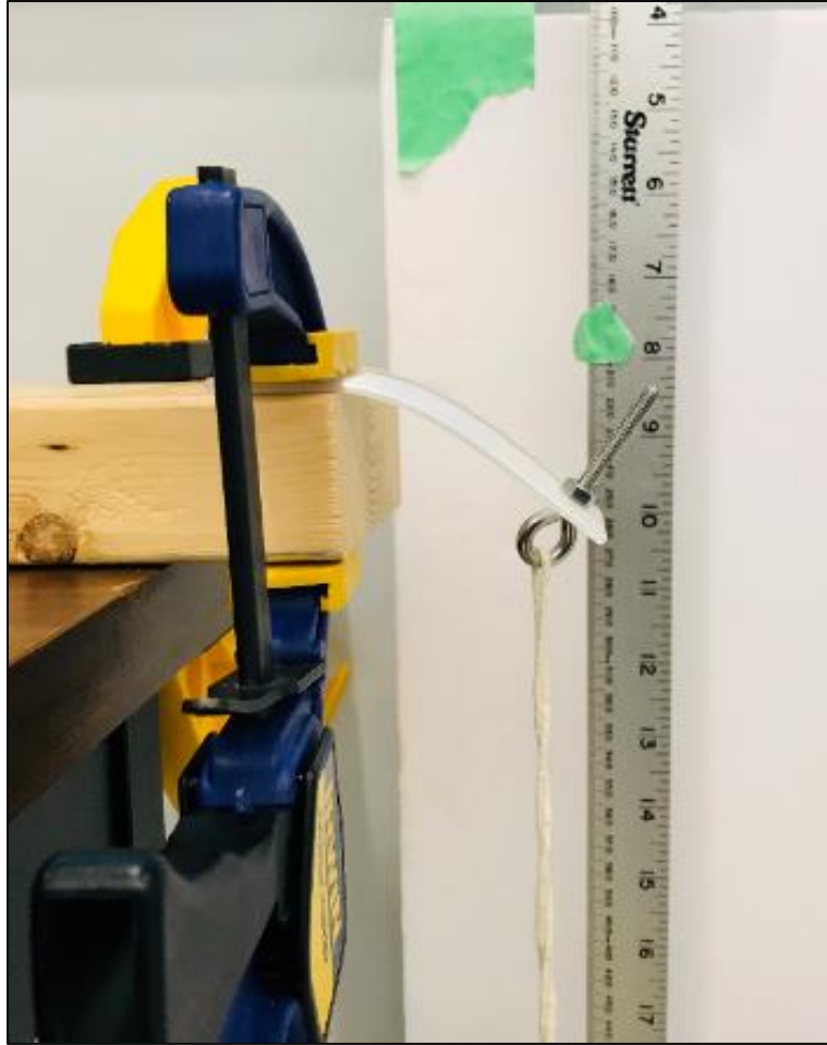
Figure 39: Position of the specimen as it is bending as the load is applied
