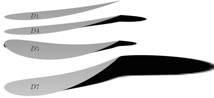
Figure 3.4: Depiction of separated flow region for ducts D1, D4, D5 and D7. The black region is where the flow is reversed
