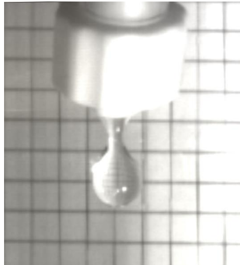
Figure 2.5: Photograph of droplet being released from release nozzle with droplet necking as critical mass surpasses droplet adhesion forces
