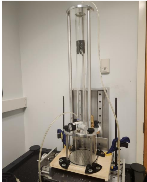
Figure 2.1: SR-TEK pressure chamber with custom droplet channel modification assembled and ready for pressurization and droplet delivery
