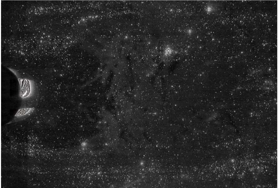
Figure 2.15 – The raw PIV image of the rotor without diffuser
