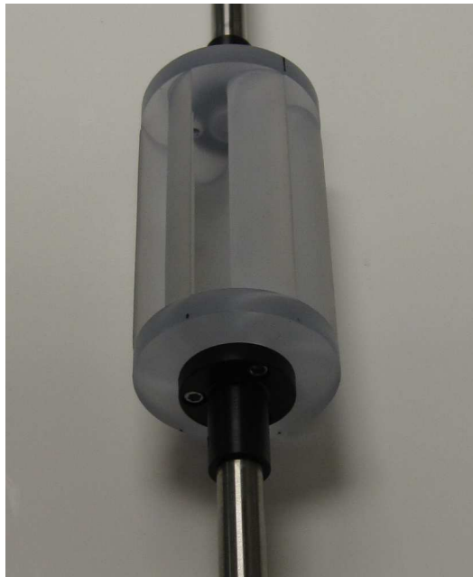
Figure 2.6 – The rotor model made by SLA technique
