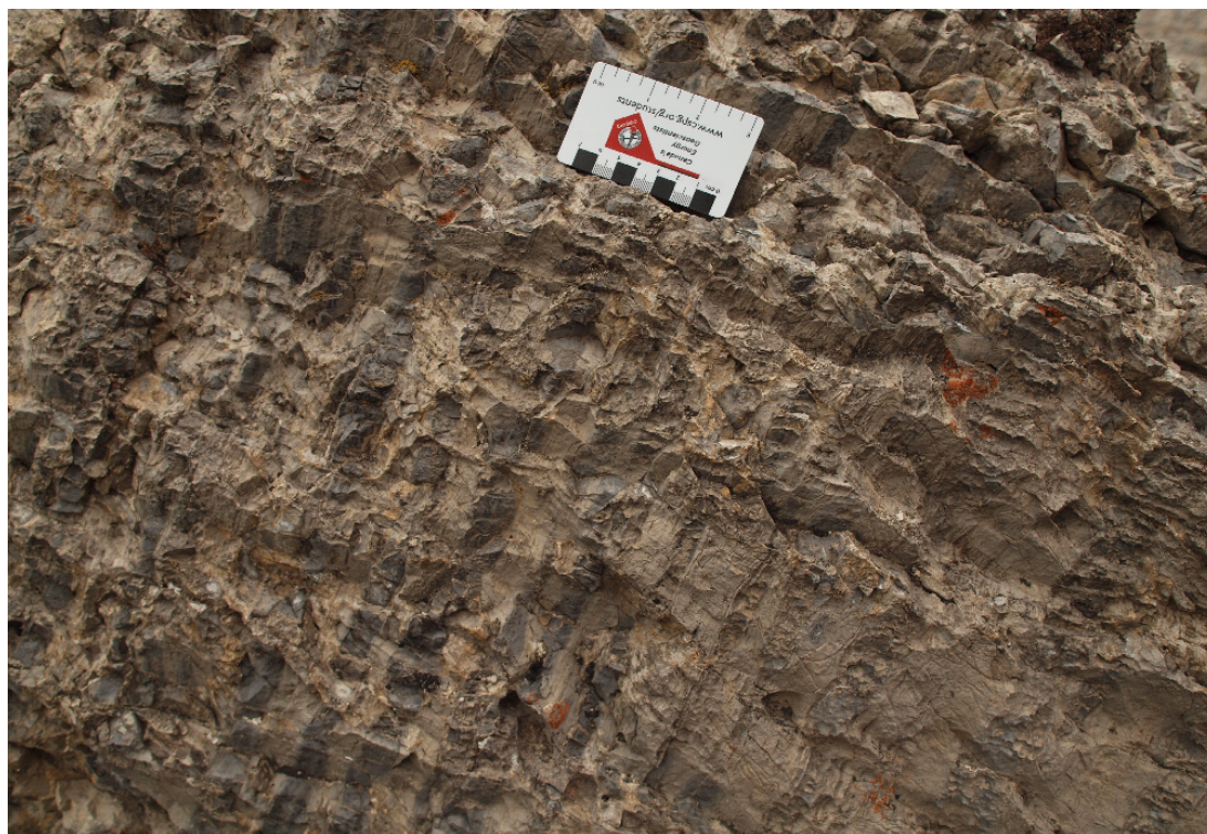
Figure 4.9: Outcrop image of lithofacies OP8 (from an outer platform environment) displaying banded layers of brown and dark brown silt. Picture of the Sassenach Formation taken at the Snaring study area.
