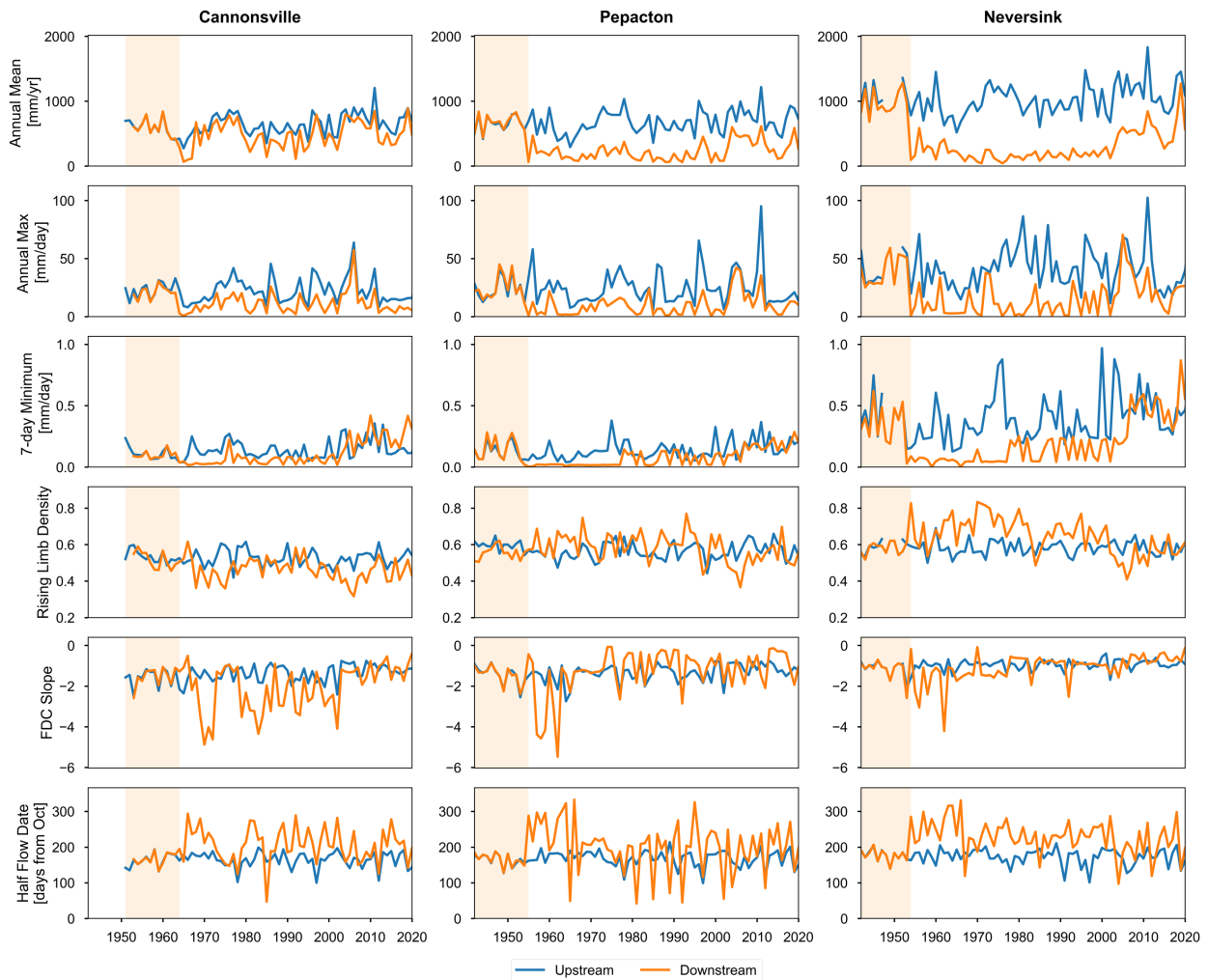
Figure 2: Time series of upstream (blue line) and downstream (orange) hydrologic signatures, where the orange shading indicates the pre-dam period for each reservoir (columns). The top row plots the annual mean streamflow [mm/year]; the second is the annual maximum daily streamflow [mm/day]; the third is the annual 7-day minimum streamflow [mm/day]; the fourth is the annual rising limb density, an indicator for flashiness; the fifth row is the slope of the flow duration curve (FDC); and the bottom row plots the mean half flow date as the number of days from October 1 st , the start of the water year.
