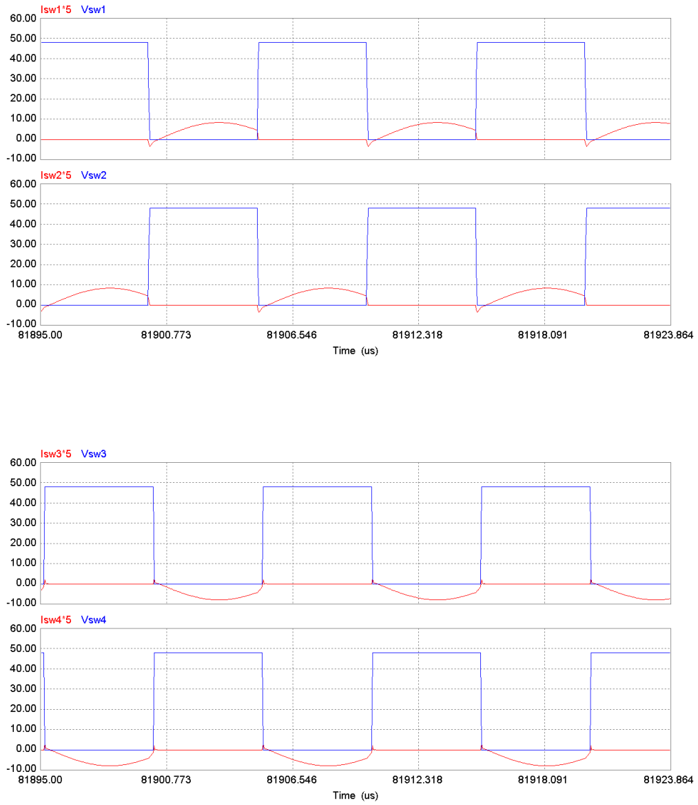
Fig. 4.19: Simulation results for DHBSRC in charging mode at 25% load with V_i = 48 V and V_o = 48 V. v_{sw1} , v_{sw2} , v_{sw3} and v_{sw4} are the switch voltages. i_{sw1} , i_{sw2} , i_{sw3} and i_{sw4} are current through switches.
