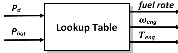
Fig 13. Pre-computed engine minimum fuel line lookup table
