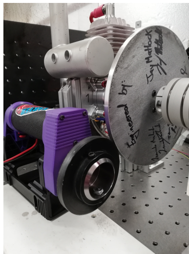
Figure 4.8: HEPS starting method of pressing hobby ICE starter against system flywheel.
