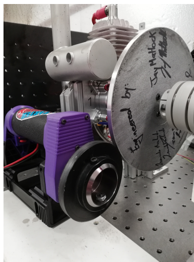
Figure 4.16: Final design for ICE starting mechanism.
