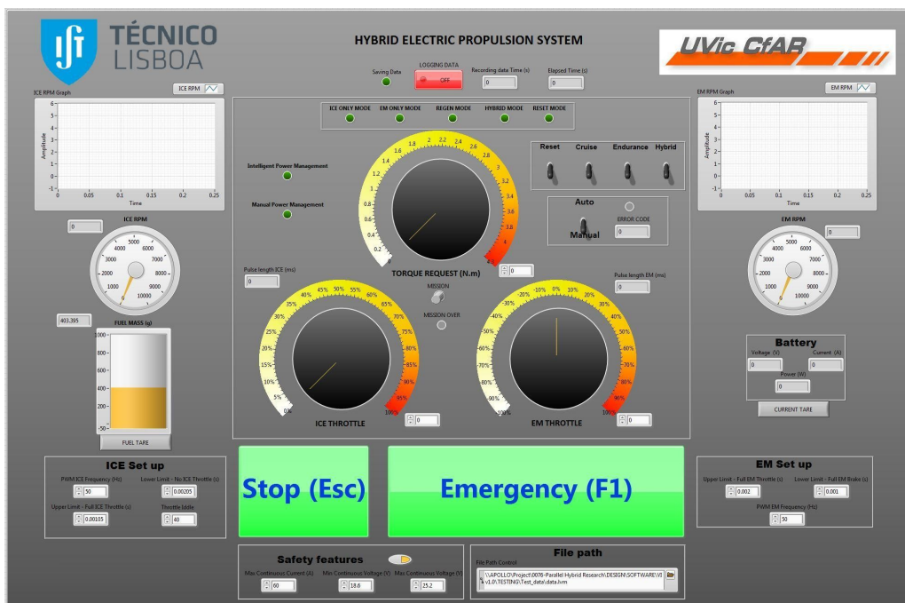
Figure 4.20: GUI developed in LabView to control and monitor performance of the parallel HEPS test bench. [63]
