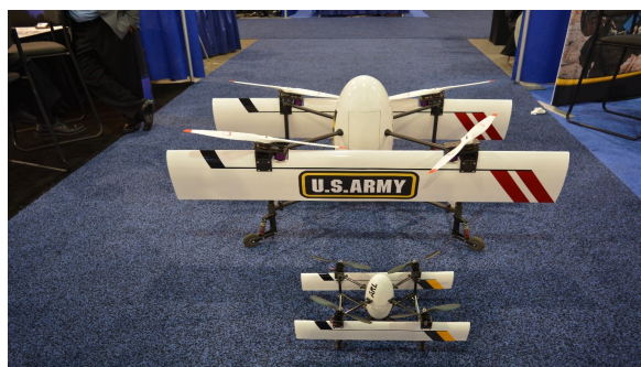
Figure 1.5: Army Research Lab's CRC-20 (top) and CRC-3 (bottom) quad-rotor biplane tailsitter UAVs.[21]
