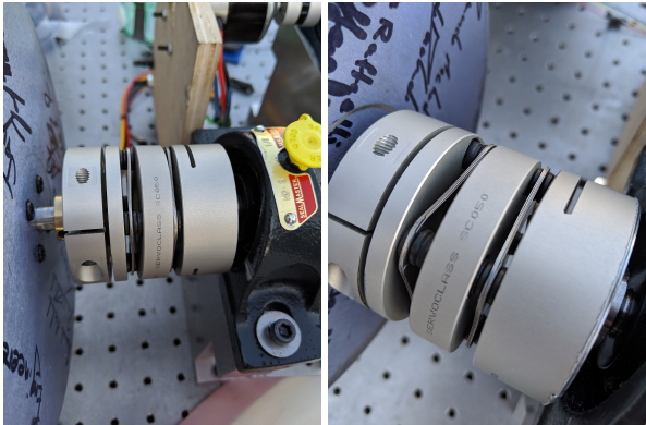
Figure 4.10: Flexible mechanical couplers used in the HEPS that clamp between shafts with metal-leaf springs.
