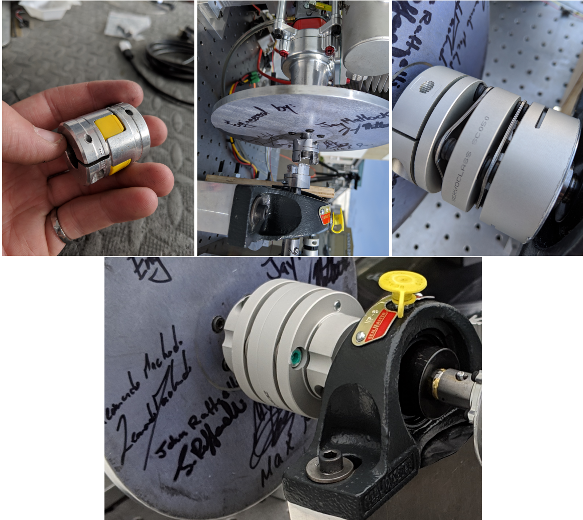
Figure A.2: Two types of mechanical couplers used in the HEPS that clamp between shafts. Rubber 'spider' coupler failed, as well as a flexible coupler with metal-leaf springs. Prevailing solution was flexible metal-leaf spring coupler with larger torque rating, as well as increased mounting stiffness to ICE.
