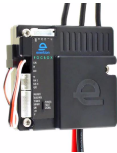
Figure 4.5: Enertion RC FOCBOX electronic speed controller capable of regenerative brake mode. [73]
