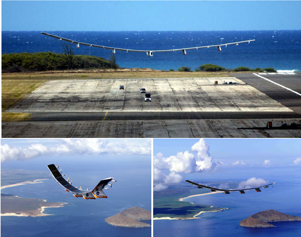
Figure 1.15: NASA Project Helios HP03-2 on Takeoff. (top) HP01 High-Altitude Configuration of NASA Project Helios. (bottom left) HP03-1 NASA Project Helios Fuel-Cell Variant flight in 2003. (bottom right) [49]
