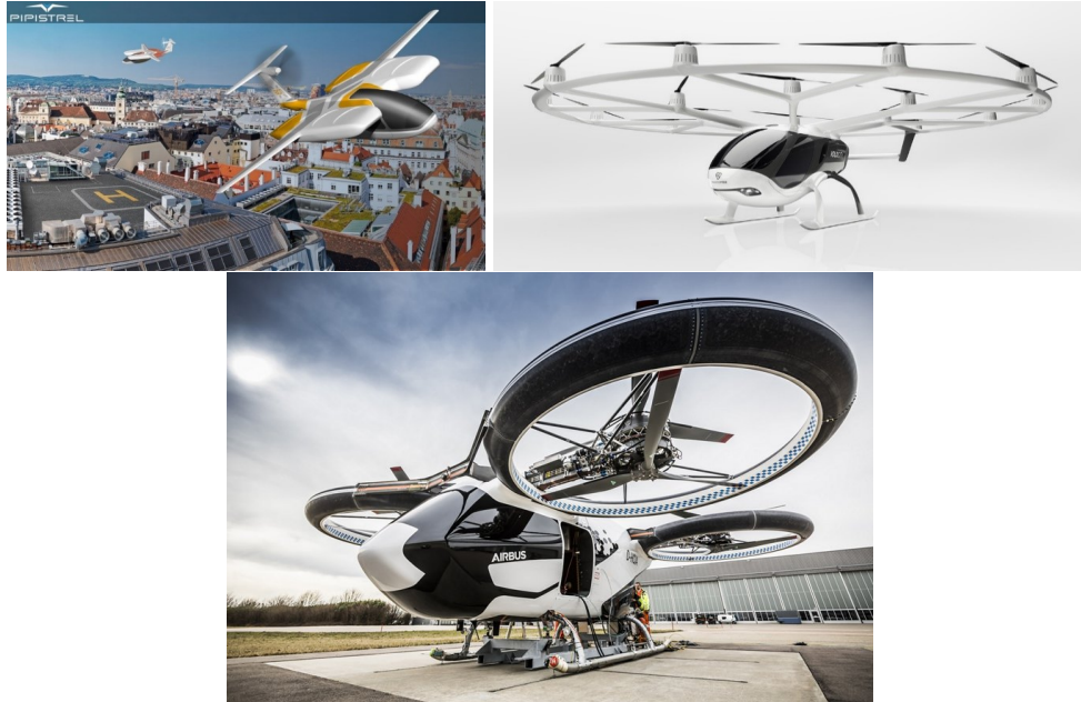
Figure 1.10: Pipistrel 801 eVTOL (top left) and Volocopter 'Volocity' (top right) and CityAirbus by Airbus A3 (bottom) UAM concepts. [34][35][36]
