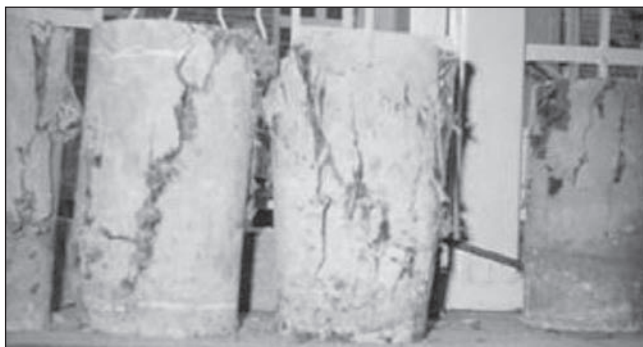
Figure 7. Bulging of cylinders during compression testing
