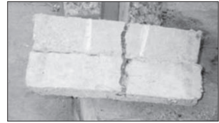
Figure 14. Beam after static flexure test
