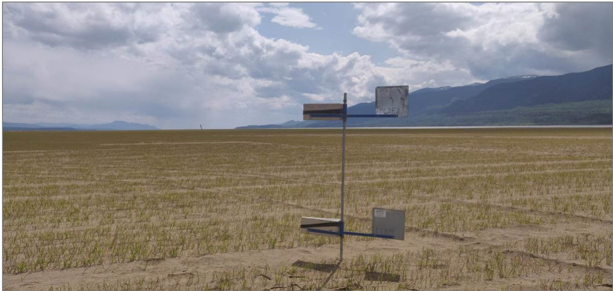
Figure 3.3: BSNE dust sampler array on MCN beach in the medium ( 200 \text{ kg ha}^{-1} ) treatment area on June 3, 2023.
