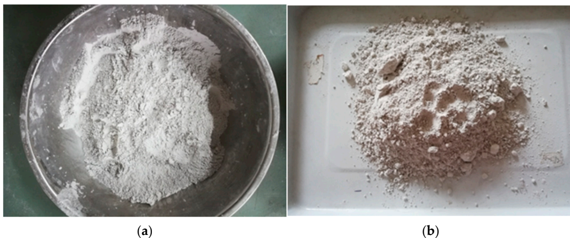
Figure 15. Raw materials. (a) UCCG (b) GGBFS powder.
