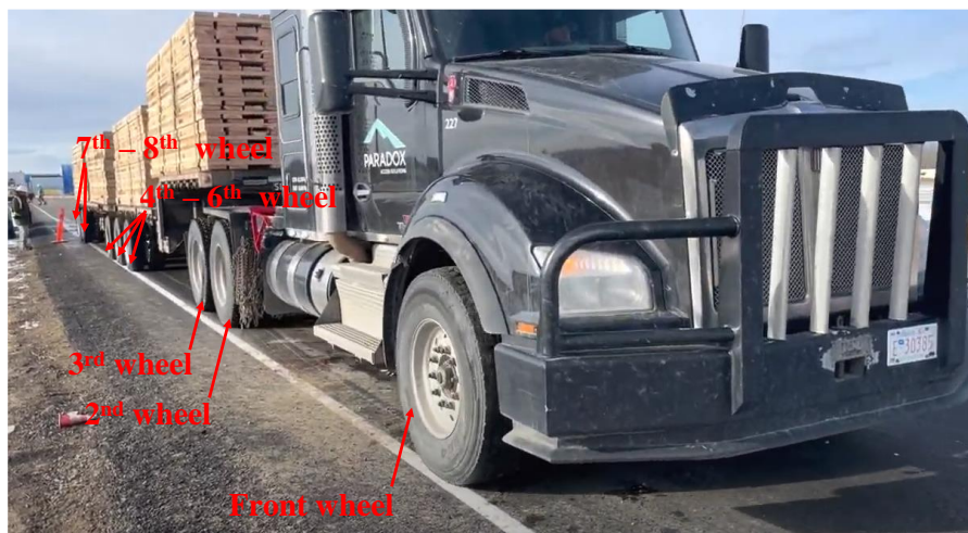
Fig. 5.29. Photograph of trafficking test on site
