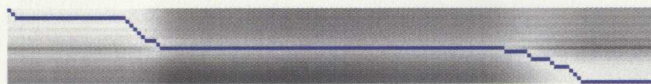
Figure 4.11: Similarity matrix visualization for the analysis of a “sit-to-stand” motion using a 20-state HMM. State values are indexed along the rows, while input frames are indexed along the columns. The Viterbi path is displayed in blue. This case demonstrates the visualization of a temporary stop in the motion.
