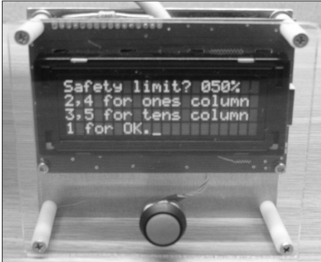
Figure 17: Tethered display and kill switch for patient.
