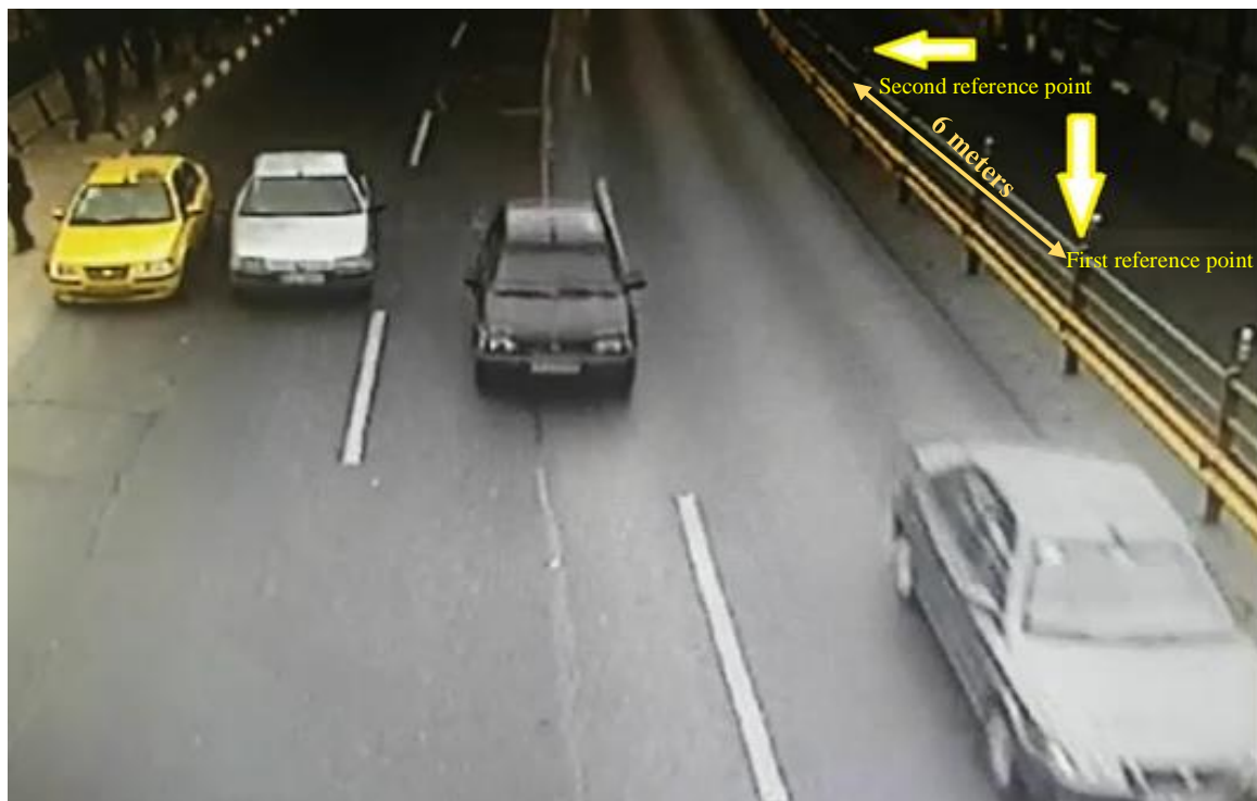
Figure 2.2: An image taken from the video data showing the two reference points.
