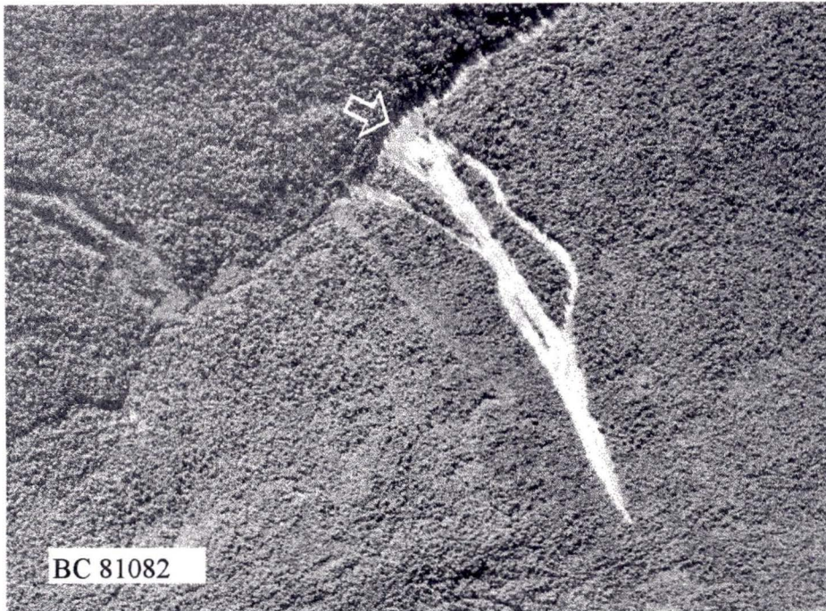
Figure 3.1: A landslide in Schmidt Creek as seen from air photograph. Note: New vegetation is beginning to grow at the base of the slide (at arrow). Original scale was 1:20,000, year was 1981.
